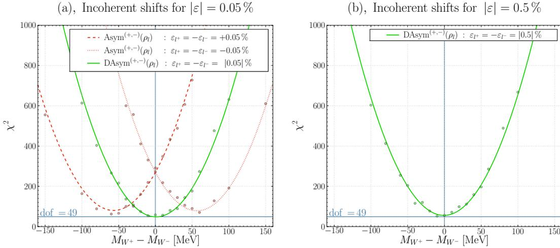
Figure 8: The  $\chi^2$  values and their polynomial fits for the incoherent shifts of the energy scale for the charge asymmetry and double charge asymmetry methods using  $|\varepsilon| = 0.05\%$  (a) and (only for the double charge asymmetry) using  $|\varepsilon| = 0.5\%$  (b).
