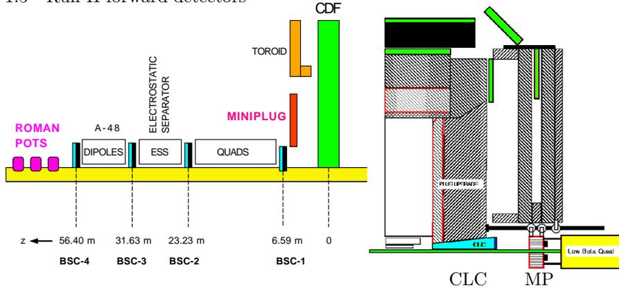
Figure 3: The CDF detector in Run II: (*left*) location of forward detectors along the  $\bar{p}$  direction; (*right*) position of the Cerenkov Luminosity Monitor (CLC) and MiniPlug calorimeters (MP) in the central detector.
