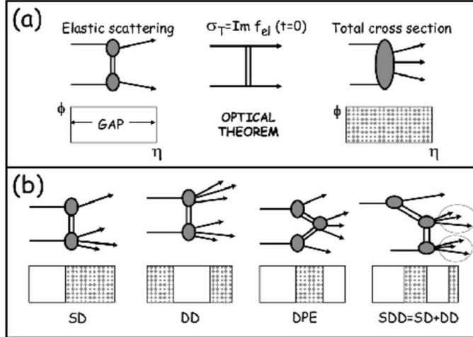
Figure 1: Schematic diagrams and event topologies in azimuthal angle  $\phi$  vs. pseudorapidity  $\eta$  for (a) elastic and total cross sections, and (b) single diffraction (SD), double diffraction (DD), double Pomeron exchange (DPE), and double plus single diffraction cross sections (SDD=SD+DD). The hatched areas represent regions in which there is particle production.
