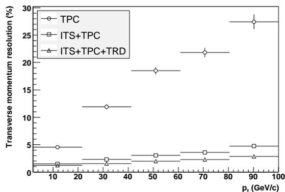
Fig. 1: Central barrel tracking resolution
