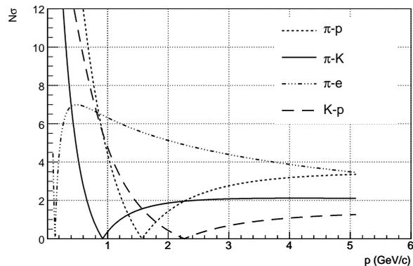
Fig. 2: Particle identification by  $dE/dx$  measurement
