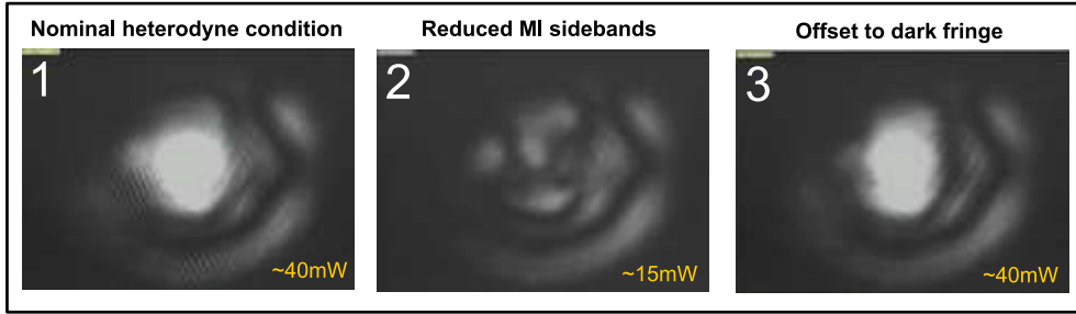
Figure 3. Realisation of DC-readout in GEO 600. Starting from a fully locked interferometer in heterodyne condition (image 1), we first turn down the RF modulation sidebands by a factor of 10 (image 2) and finally introduce a dark-fringe offset that couples TEM 00 carrier light into the output port, serving as new local oscillator (image 3).
