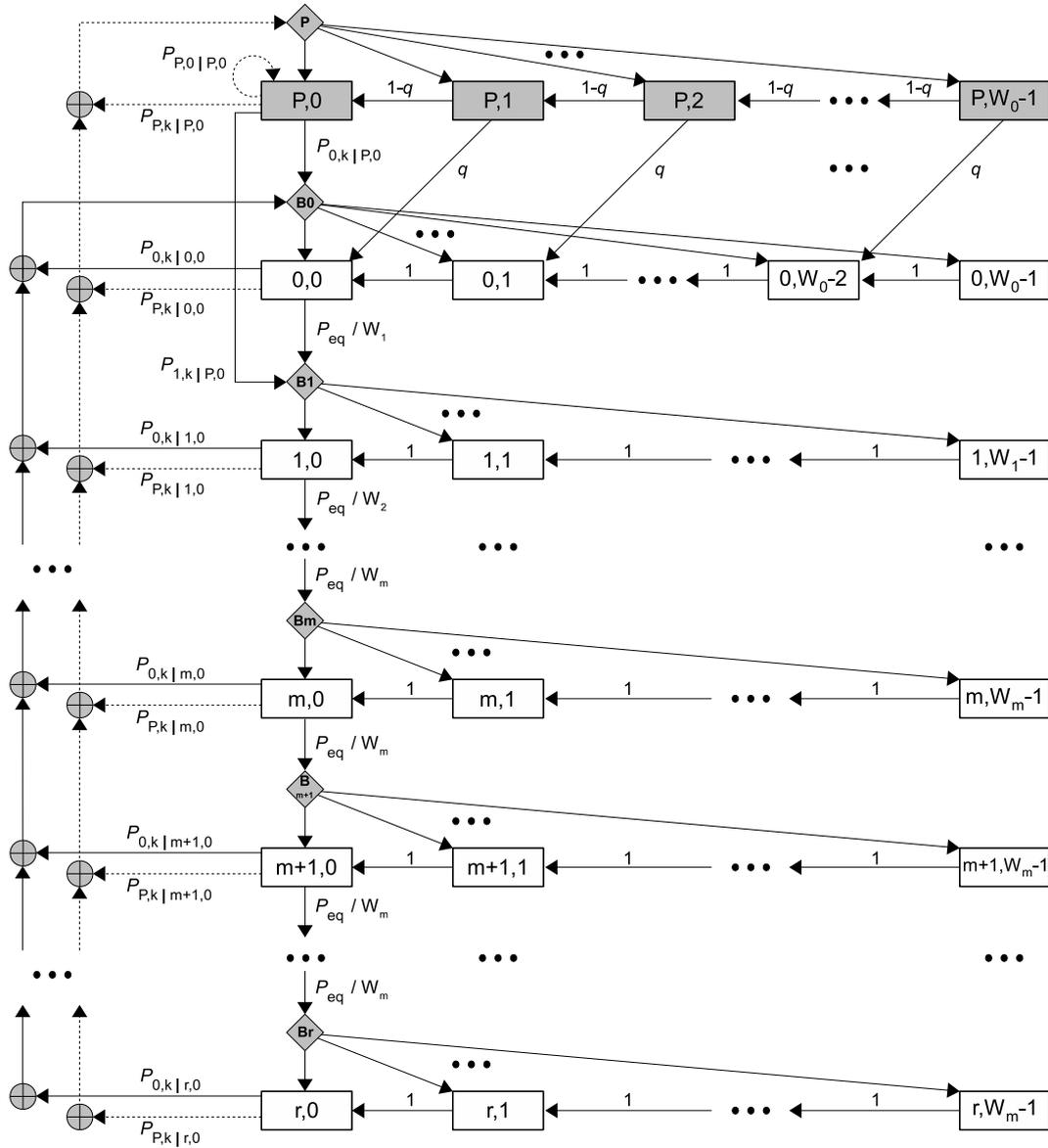
Fig. 1. Markov chain for the contention model of the generic  $s$ -th station in general traffic conditions, based on the 2-way handshaking technique, considering the effects of channel induced errors, unloaded traffic conditions, and post-backoff.
