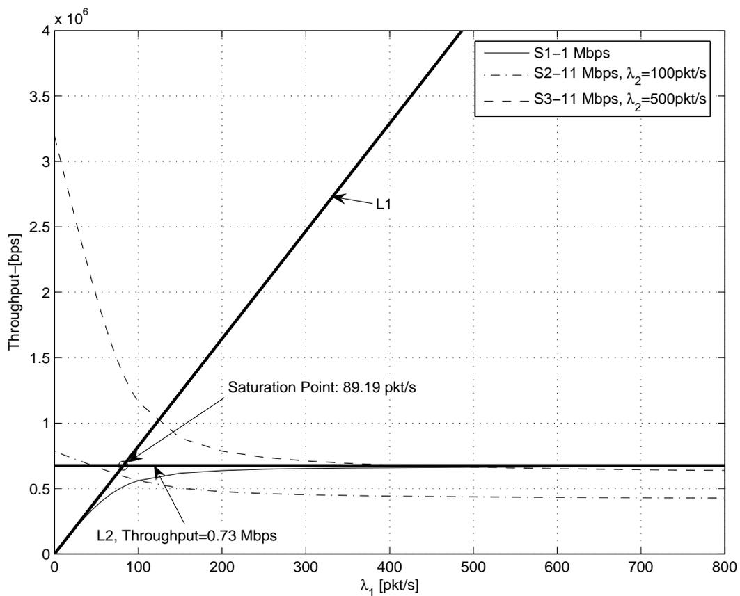
Fig. 3. Behaviour of the per-station throughput in a network of three contending stations (labelled S1, S2 and S3) as a function of the packet rate  $\lambda_1$  of the slowest station S1 transmitting at 1 Mbps. The other two stations transmit at 11 Mbps with constant packet rates, respectively equal to 100pkt/s and 500pkt/s. The packet size PL is equal to 1028 bytes for the three contending stations.
