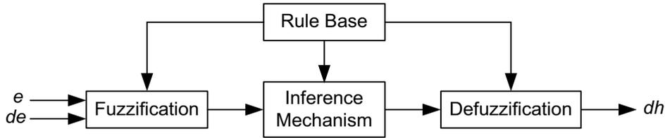
**Figure 3.** Inner structure of fuzzy logic controller.
