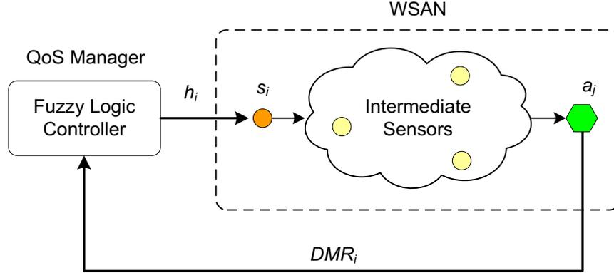
**Figure 2.** Fuzzy logic control based QoS management.
