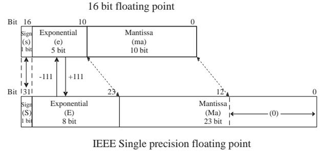
Fig. 7. Conversion between 16-bit floating point and IEEE single precision floating point.
