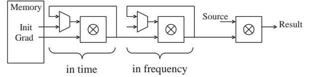
Fig. 16.  $\Delta W$  correction circuit.
