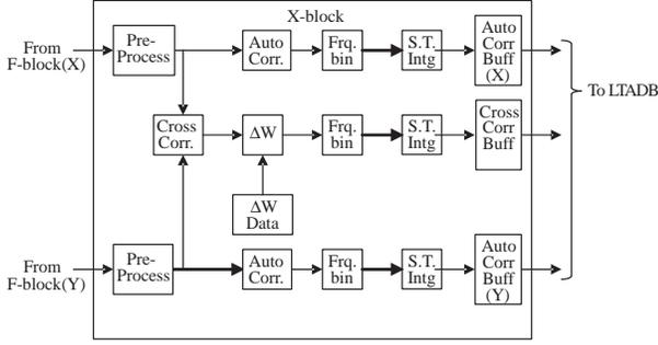
Fig. 13. Block diagram of the correlation in a FX mode.
