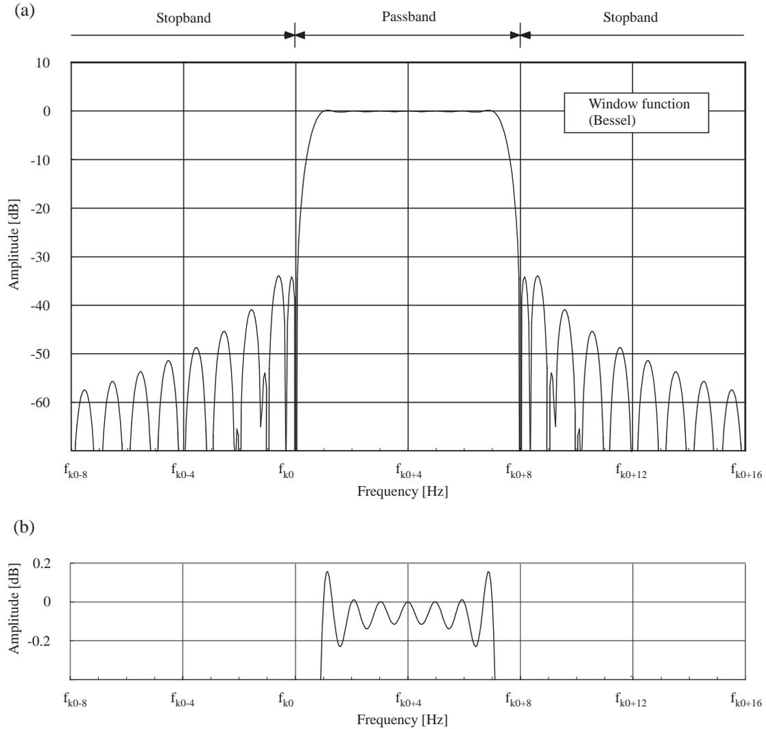
**Fig. 2.** The frequency response of 1st FFT stage in the FFX scheme, which works as a digital filter. (a) is the frequency response at the full range to investigate the stopband, and (b) is the closeup frequency response in the passband to investigate a ripple. The frequency response is multiplied by the window of the Bessel function,  $w(n) = J_0\left(\frac{4.24n}{N_n}\right)$ .
