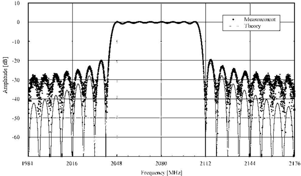
**Fig. 20.** The measured frequency response of the FFX correlator at a bandwidth of 64 MHz in a frequency range of 2048 to 2112 MHz. First sidelobe of about  $-20$  dB and other stopband response of better than  $-23$  dB were successfully achieved. A comparison between the measured frequency response of the FFX correlator (points) and the ideal frequency response of the FFX scheme (full line) in a rectangular window function without zeroing [see equations (14) and (11)] are shown.
