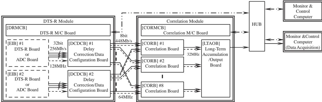
Fig. 3. Correlation processing block diagram of the FFX scheme.
