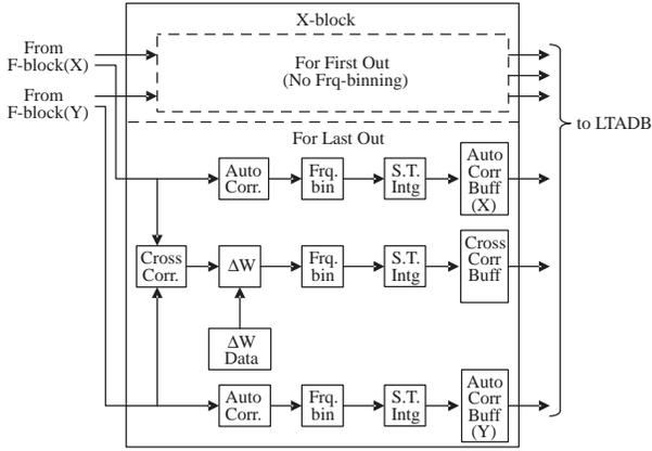
Fig. 14. Block diagram of the correlation in a FFX mode.
