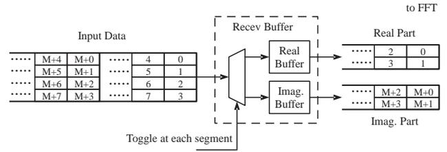
Fig. 8. Parallel processing of two datasets in FFT.
