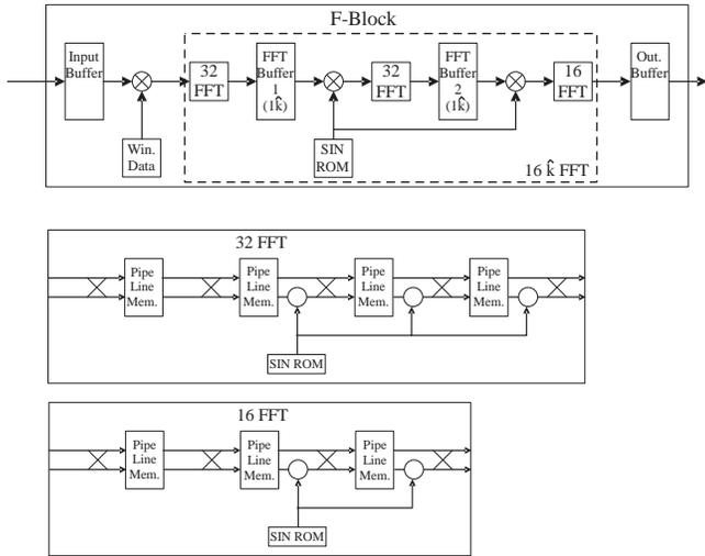
**Fig. 9.** Pipeline processing of the FX scheme ( $16\hat{k}$ -point FFT).
