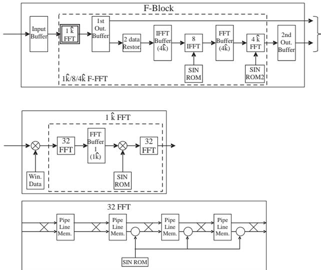
**Fig. 10.** Pipeline processing of the FFX scheme ( $1\hat{k}$ -point FFT, 8-point IFFT,  $4\hat{k}$ -point FFT).
