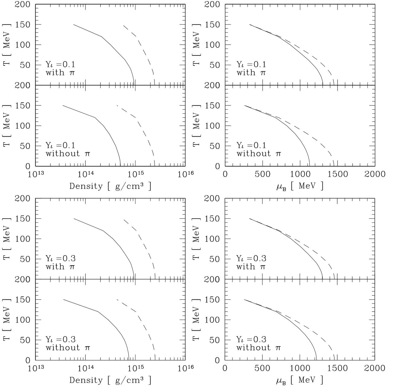
FIG. 5: Phase diagrams of our EOS of the SN matter with  $Y_l = 0.1$  and  $0.3$  for  $T < 150$  MeV. Solid lines represent boundaries of hadronic matter and mixed matter and dashed lines do those of mixed matter and quark matter. For the upper plots in each panel, an EOS with pions is used while an EOS without pions is used for the lower plots in each panel.  $B = 250 \text{ MeV fm}^{-3}$  is chosen for the bag constant for all panels.
