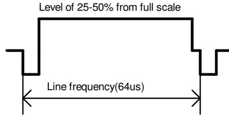
Fig.1.Waveform used for the noise performance evaluation
