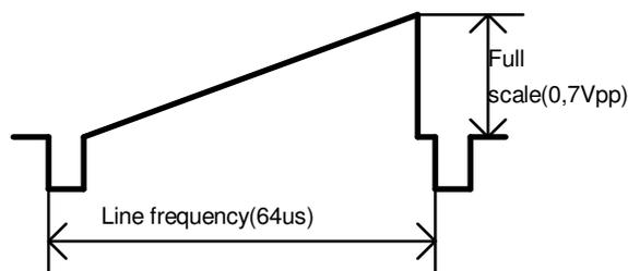
Fig.2.Waveform used for ADC parameters evaluation
