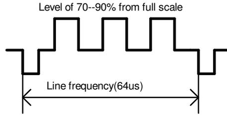
Fig.3.Waveform used for Synchronisation accuracy test
