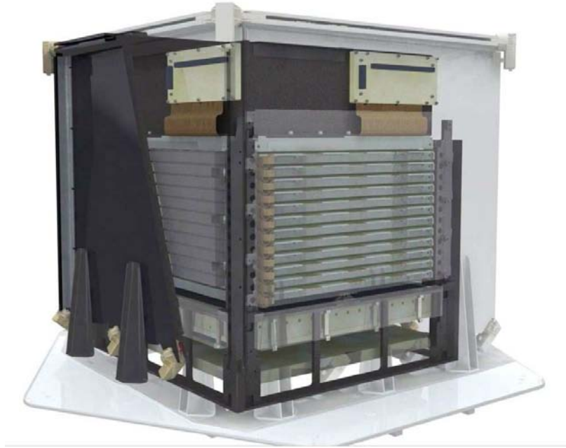
Figure 2: The AGILE scientific instrument showing the hard X-ray imager, the gamma-ray Tracker, and Calorimeter. The Anticoincidence system is partially displayed, and no lateral electronic boards and harness are shown for simplicity. The AGILE instrument "core" is approximately a cube of about 60 cm size and of weight equal to 100 kg.
