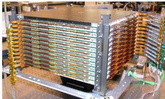
Figure 2: The silicon tracker before the integration with the payload and the flight DAQ (June 2005)
