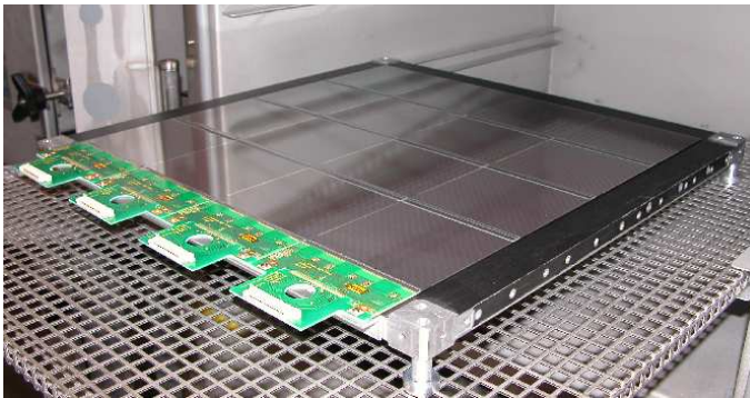
Figure 7: A tray with the four ladders glued on one of the views.
