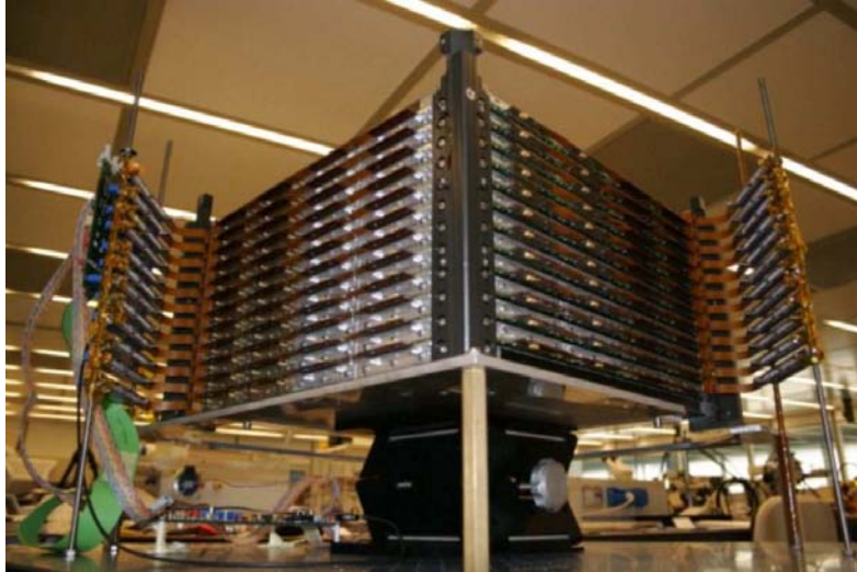
Figure 4: The assembled AGILE Silicon Tracker developed by the INFN laboratories of Trieste before being integrated with the rest of the instrument (June 2005).
