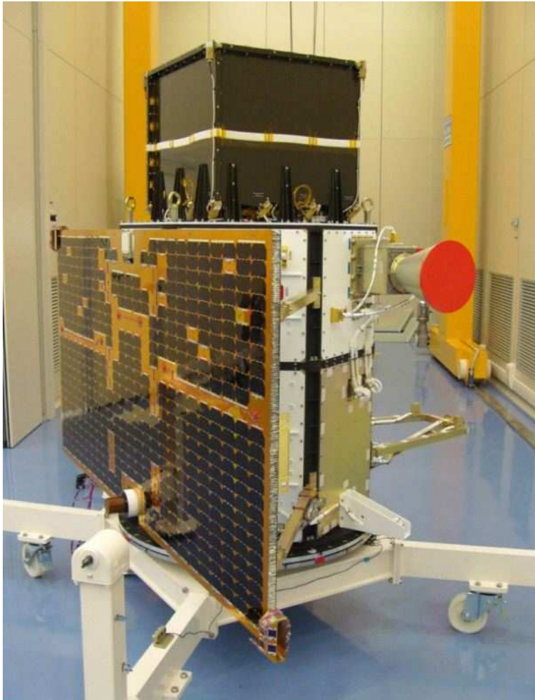
Figure 3: The integrated AGILE satellite in its final configuration before being covered by the thermal blanket. The total satellite mass is equal to 350 kg.
