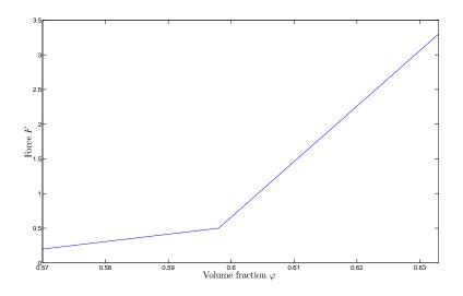
Figure 1.  $F(\varphi)$  versus  $\varphi$  given by (5) with  $\varphi_c = .598$ ,  $F(\varphi_c) = .5$ ,  $\alpha = 10.7$  and  $\beta = 80$ . These values were chosen to make the graph resemble that in Figure 2 of [1], which shows the force  $F(\varphi)$  in newtons versus the volume fraction  $\varphi$  for a penetration depth of 60mm.
