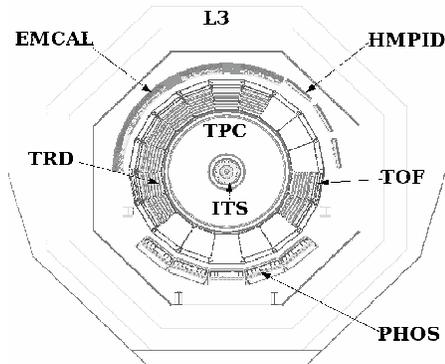
Fig. 1. Sketch of the ALICE experiment, transverse view.
