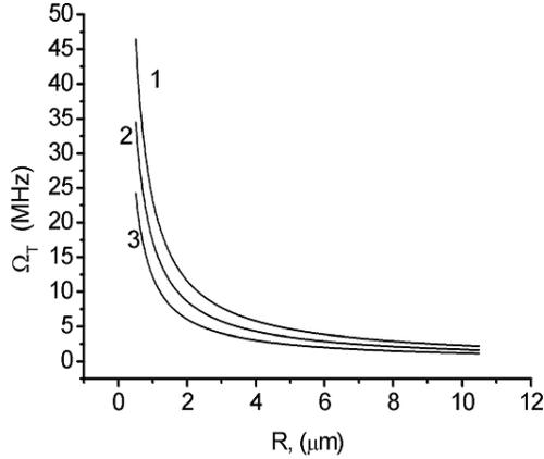
FIG. 6: The thermal combination anti-Stokes frequency of LITS for fused silica microsphere  $Q_f = 10^7$ ,  $\lambda_p = 1.550 \mu m$ , 1.  $TE_{230}^1 - T_1^0$ , 2.  $TE_{170}^1 - T_1^0$ , 3.  $TE_{120}^1 - T_1^0$ .
