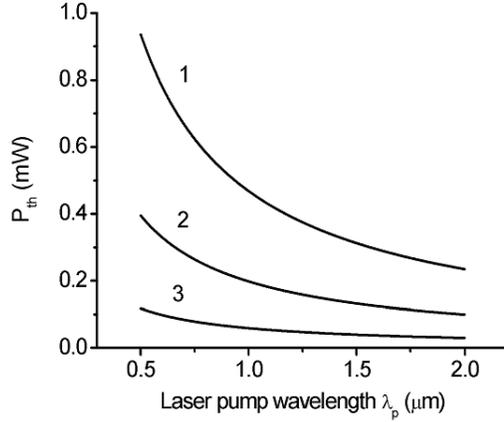
FIG. 1: The threshold power of LITS depends on resonant wavelength of wide range of gas laser and solid state semiconductor lasers. Radius of fused silica microsphere: 1.  $R = 20 \mu m$ , 2.  $R = 15 \mu m$ , 3.  $R = 10 \mu m$ ,  $Q_f = 10^8$ ,  $TE_n^1 - T_1^1, n \approx \rho$ .
