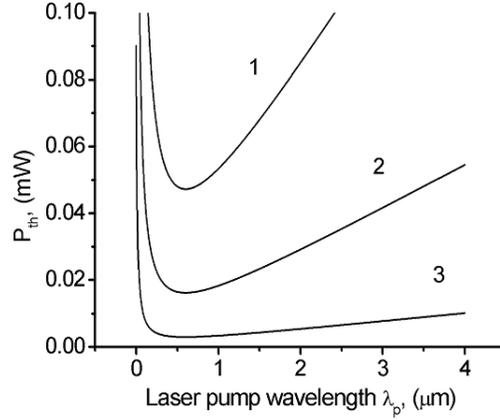
FIG. 4: The minimum of threshold of LITS for silica microsphere at the laser pump  $\lambda_p = 0.532 \mu m$  with radii 1.  $R = 70 \mu m$ , 2.  $R = 45 \mu m$ , 3.  $R = 50 \mu m$ .
