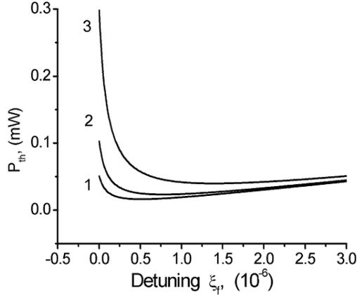
FIG. 2: The threshold power of LITS as a function of detuning  $\xi_f$  (radius  $R = 35 \mu m$ ) exited the MDR's: 1.  $\lambda_p = 0.532 \mu m$ ,  $TE_{600}^1 - T_1^0$  modes, 2.  $\lambda_p = 0.840 \mu m$ ,  $TE_{300}^1 - T_1^0$  modes. 3.  $\lambda_p = 1.55 \mu m$ ,  $TE_{210}^1 - T_1^0$ .
