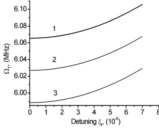
FIG. 3: The thermal combination anti-Stokes frequency of LITS as a function of detuning  $\xi_f$  (radius  $R = 35 \mu m$ ) exited the MDR's: 1.  $\lambda_p = 0.532 \mu m$ ,  $TE_{600}^1 - T_1^0$  modes, 2.  $\lambda_p = 0.840 \mu m$ ,  $TE_{300}^1 - T_1^0$  modes. 3.  $\lambda_p = 1.55 \mu m$ ,  $TE_{210}^1 - T_1^0$ .
