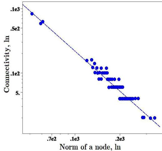
Figure 5: The scatter plot of the connectivity vs. the norm a node in the dual graph representation of 96 Venetian canals acquires with respect to random walks. Three data points characterized by the shortest access times represent the main water routes of Venice: the Lagoon of Venice, the Giudecca canal, and the Grand canal. Four data points of the worst accessibility are for the canal subnetwork of Venetian Ghetto. The slope of the regression line equals 2.07.
