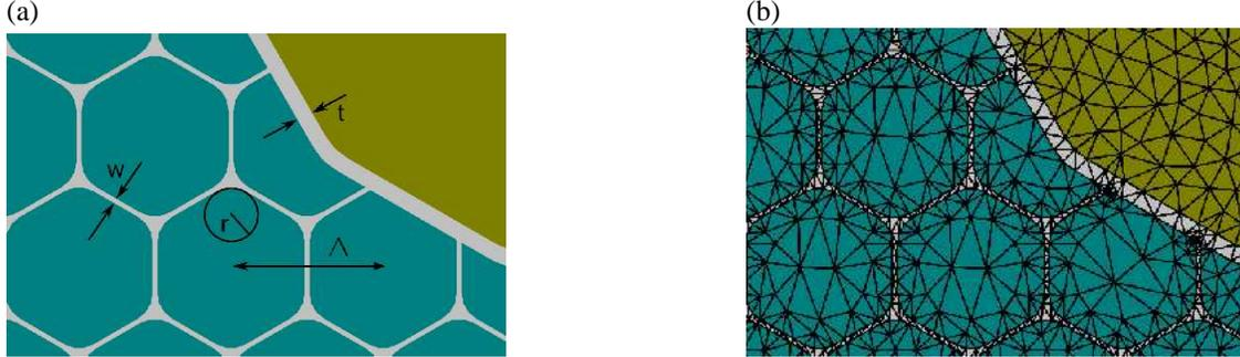
**Fig. 7** (a) geometrical parameters describing HCPCF: pitch  $\Lambda$ , hole edge radius  $r$ , strut thickness  $w$ , and core surround thickness  $t$ ; (b) detail from a triangulation of HCPCF. Due to the flexibility of triangulations all geometrical features of the HCPCF are resolved.
