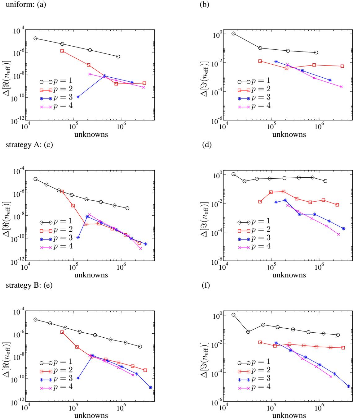
**Fig. 4** Relative error of fundamental eigenvalue in dependence on number of unknowns of FEM computation for different refinement strategies and finite element degrees  $p$ . Parameters:  $\Lambda = 1550$  nm,  $r = 300$  nm,  $w = 50$  nm,  $t = 170$  nm, 6 cladding rings, wavelength  $\lambda = 589$  nm. Adaptive refinement strategy A minimizes residuum (26), strategy B minimizes residua (26) and (27)
