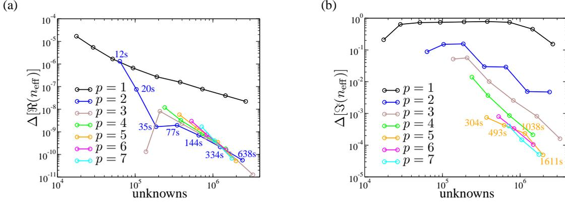
**Fig. 6** Relative error of fundamental eigenvalue in dependence on number of unknowns of FEM for adaptive refinement and different finite element degrees  $p$ . Parameters:  $\Lambda = 1550$  nm,  $r = 300$  nm,  $w = 50$  nm,  $t = 170$  nm, 6 cladding rings, wavelength  $\lambda = 600$  nm. Computational times are shown.
