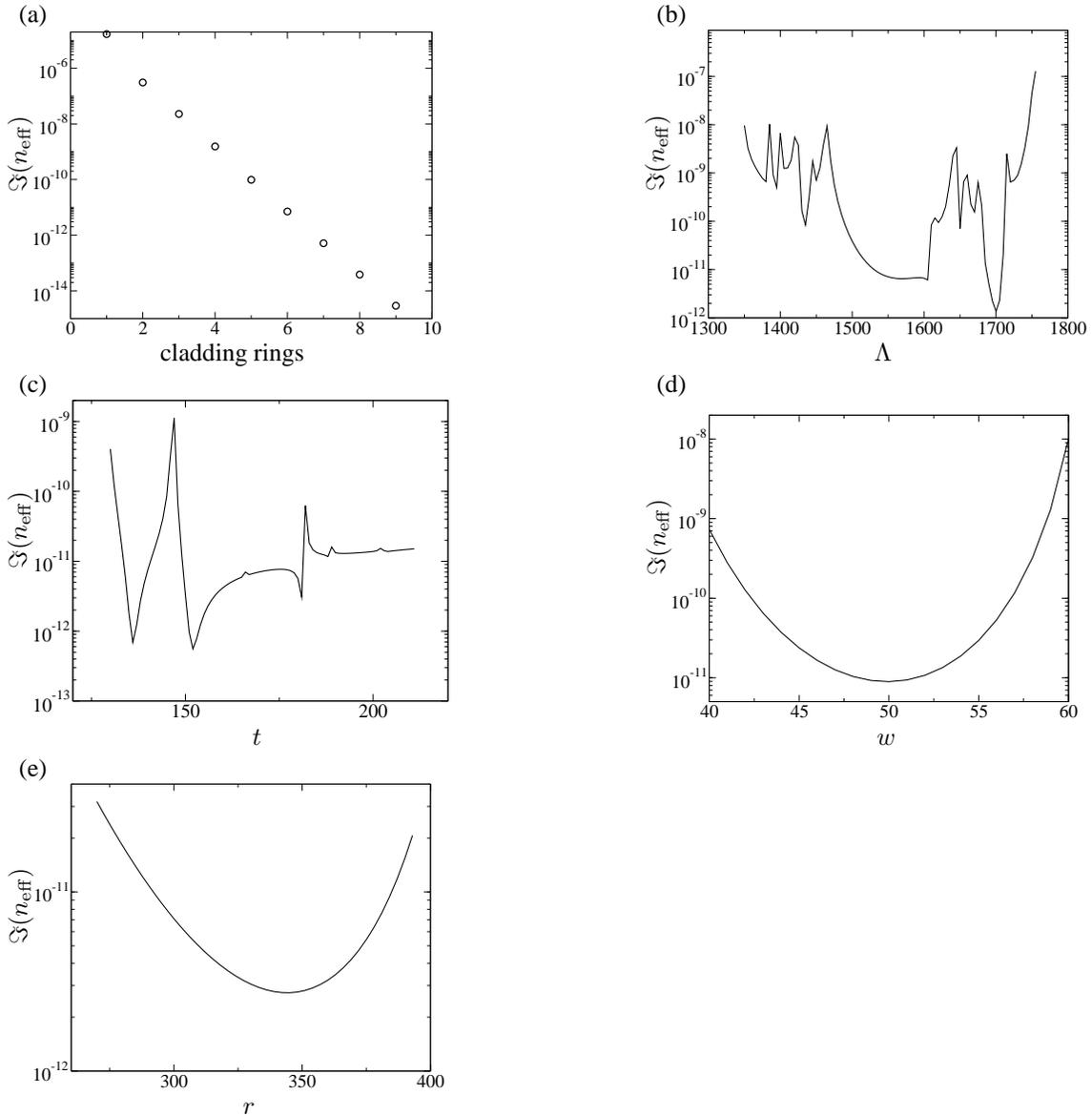
**Fig. 8** Imaginary part of effective refractive index  $\Im(n_{\text{eff}})$  in dependence on: (a) number of cladding rings, (b) pitch  $\Lambda$ , (c) core surround thickness  $t$ , (d) strut thickness  $w$ , (e) hole edge radius  $r$ . Parameters:  $\Lambda = 1550$  nm,  $r = 300$  nm,  $w = 50$  nm,  $t = 170$  nm, 6 cladding rings, wavelength  $\lambda = 589$  nm.
