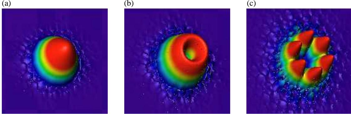
**Fig. 2** First, second and fourth fundamental core modes of HCPCF illustrated in Fig. 3(a) - Parameters:  $\Lambda = 1550$  nm,  $r = 300$  nm,  $w = 50$  nm,  $t = 170$  nm,  $\lambda = 589$  nm, see Fig. 7(a) for definition of parameters.
