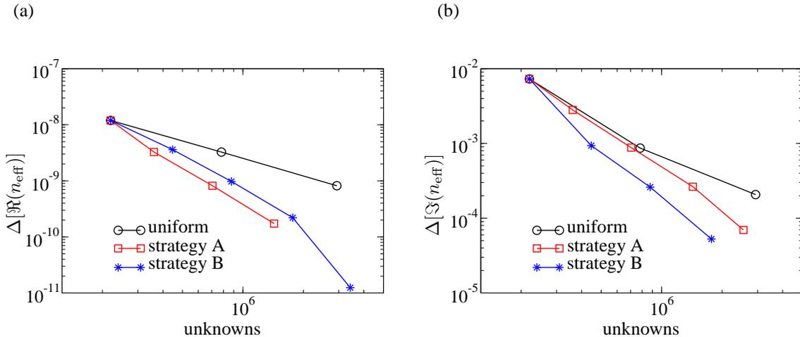
**Fig. 5** Relative error of fundamental eigenvalue in dependence on number of unknowns of FEM computation for different refinement strategies and finite element degree  $p = 3$ . Parameters:  $\Lambda = 1550$  nm,  $r = 300$  nm,  $w = 50$  nm,  $t = 170$  nm, 6 cladding rings, wavelength  $\lambda = 589$  nm. (a) uniform refinement, (b) adaptive refinement, (c) goal-oriented refinement
