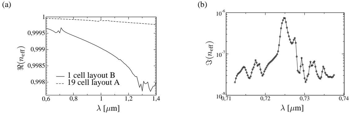
**Fig. 10** (a) Real part of effective refractive index of fundamental leaky mode in dependence on wavelength  $\lambda$  for 19-cell and 1-cell kagome-structured fiber. Parameters: see Table 2 - (b) zoom into Fig. 11(a).
