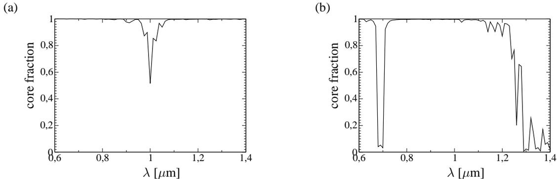
**Fig. 13** (a) Fraction of electric field intensity of fundamental leaky mode located inside hollow core in dependence on wavelength  $\lambda$  for (a) 19-cell and (b) 1-cell kagome-structured fiber. Parameters: see Table 2
