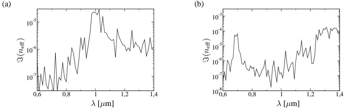
**Fig. 11** Imaginary part of effective refractive index of fundamental leaky mode in dependence on wavelength  $\lambda$  for (a) 19-cell and (b) 1-cell kagome-structured fiber. Parameters: see Table 2
