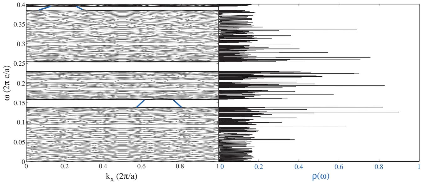
FIG. 2: *Left*: Frequency spectrum  $\omega$  of the Fibonacci quasicrystal vs. “wave-vector”  $k_x$ . The blue lines indicate spurious states which arise due to finite resolution effects (see text). *Right*: Corresponding density of states  $\rho(\omega)$  computed using a transfer-matrix technique with a supercell of  $10^4$  layers. *Inset*: Power distribution  $\sim |H_z|^2$  (red/white = positive/zero) of a spurious state, the field profile of which oscillates at the Nyquist frequency.
