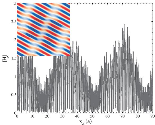
FIG. 4: Plot of the magnetic field amplitude  $|H_z|$  for a band-edge state taken along a slice of the two-dimensional superspace (in the  $\phi$  direction). *Inset*: Two-dimensional superspace field profile (red/white/blue indicates positive/zero/negative amplitude).
