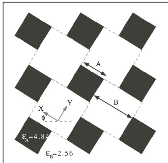
FIG. 1: Unit cell of the Fibonacci superspace dielectric. The physical dielectric is obtained by taking a slice at an angle  $\tan \phi = \tau$ . Black/white are the dielectric constants of the structure factor material and air, chosen to be  $\epsilon = 4.84$  and  $\epsilon = 2.56$ , respectively.
