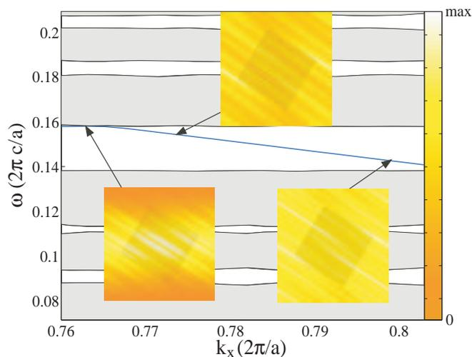
FIG. 3: Enlarged view of the Fibonacci spectrum showing a gap with a spurious band crossing it. Insets show the magnetic field  $|H_z|$  for the spurious band at various  $k_x$ —the localization of this mode around the  $X$ -parallel edges of the dielectric indicate that this is a discretization artifact.
