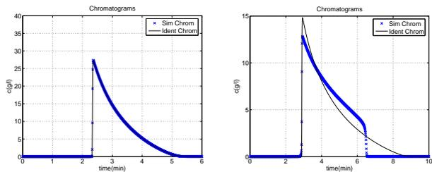
(a) Simulation using a Langmuir isotherm, identification using a Langmuir model: the chromatogram is perfectly fit. (b) Simulation using a Lattice isotherm, identification using a Langmuir model: poor fit of the chromatogram.
