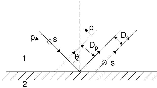
Fig. 1. Geometry indicating the GH shift, defined as  $D$ . A beam of light with a finite transverse extent is incident from vacuum (medium 1) on a metal surface (medium 2). If the beam is  $s$  polarized, the displacement of the reflected beam (dotted line) with respect to the geometrical reflection (continuous line) is positive. If the beam is  $p$  polarized, the displacement is negative.
