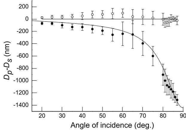
Fig. 5. Measured Goos-Hänchen shifts, i.e. the difference between  $D_p$  and  $D_s$  as a function of the angle of incidence. Experimental data are shown as solid dots and the corresponding theoretical curve has been derived from Fig. 2. The open dots show displacements orthogonal to the plane of incidence; the theoretical line in this case indicates zero displacement.
