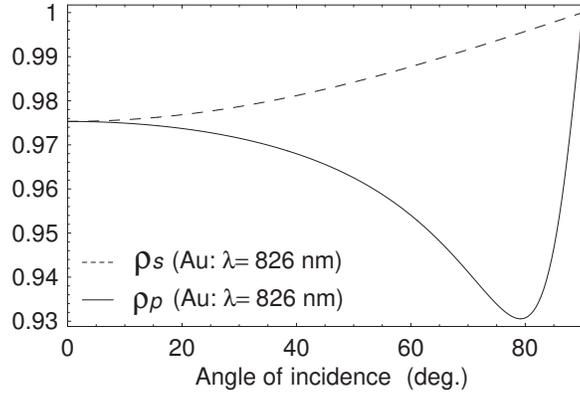
Fig. 4. Calculated reflectivity of Au at a wavelength of 826 nm, as a function of the angle of incidence. We verified experimentally that the difference in the reflectivity for the  $s$  and  $p$  polarized beams is maximal at  $80^\circ$ .
