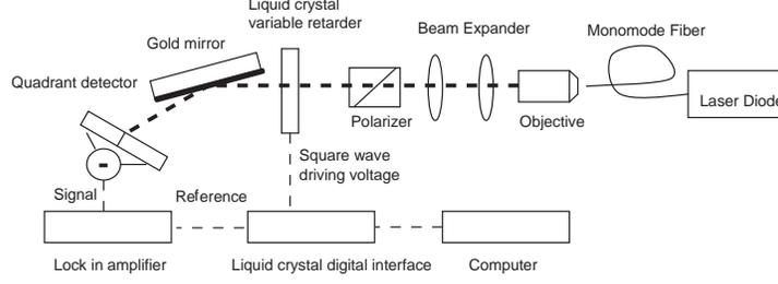
Fig. 3. Schematic drawing of the experimental set up.
