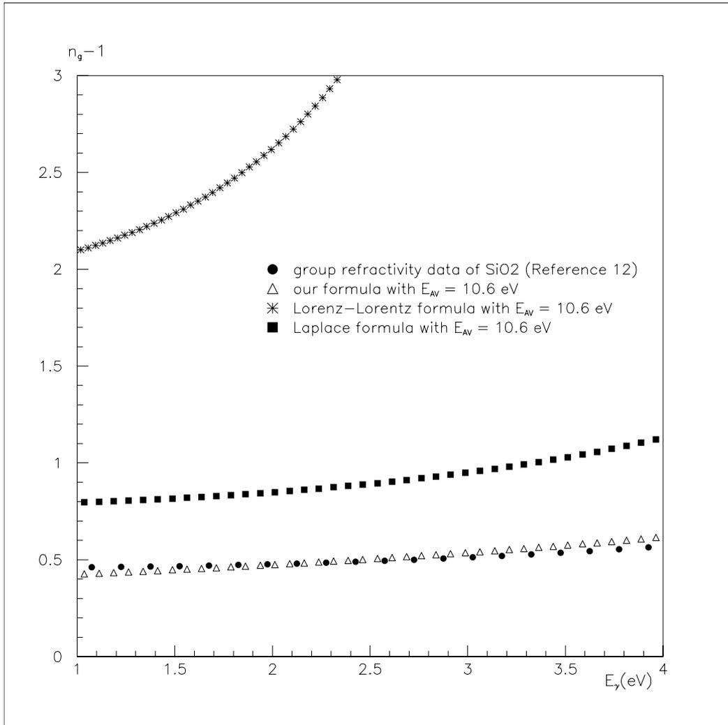
Figure 2. The fused silica group refractivity: n<sub>g</sub>-1, as a function of the photon energy in eV.
