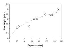
Figure 2 : Finite element simulation compared to measured data
