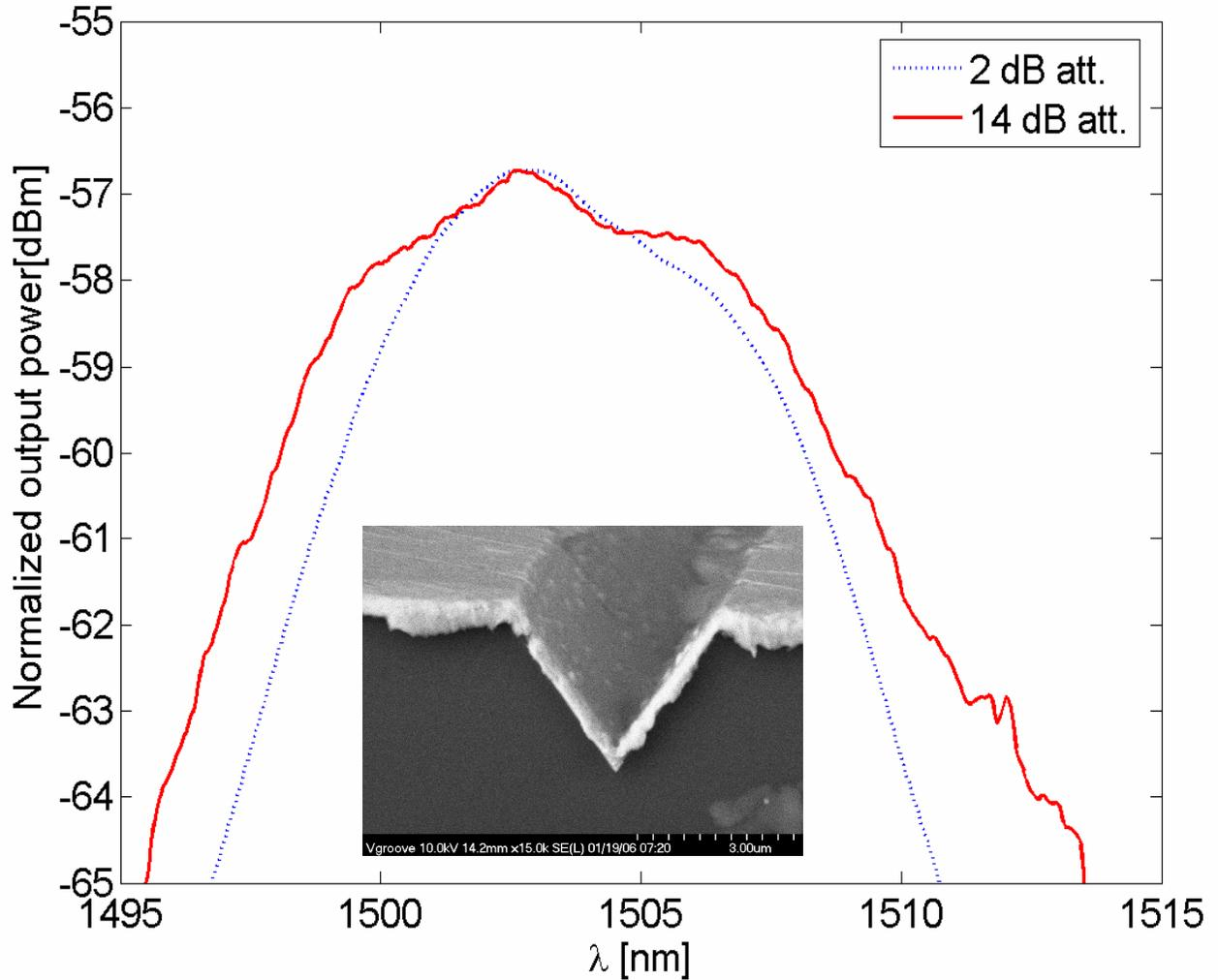
**Fig.3. Intensity dependent spectrum of v-groove plasmonic waveguide.**
