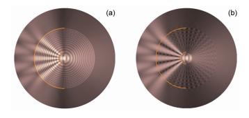
Fig. 4. (Color online) Magnitude of H-field calculated with non-magnetic design rules of Eqs. (6) and (7). Orange curves indicate input and output arcs for Fig. 3b. Both designs use  $a=600\,\mathrm{nm}$ ,  $b=610\,\mathrm{nm}$ , and  $l=3\,\mathrm{\mu m}$ , with the test sources of Fig. 2. (a) Impedance is matched at the internal interface,  $\rho=a$ , the design rules of Eq. (6) are used. (b) Impedance is matched at the external interface,  $\rho=l$ , using the rules of Eq. (7).
