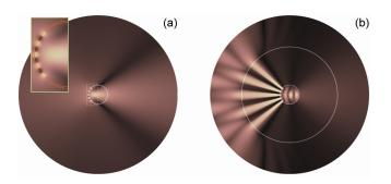
Fig. 2. (Color online) Numerical simulations of the ideal lens. (a) H-field magnitude generated by test sources in free space. Inset: five test sources at a virtual circumference,  $\rho=a-30~\mathrm{nm}$ . (b) Imaging of the same sources using an ideal hyper-lens with the design rules of Eq. [5] and matched impedance at the internal boundary,  $\rho=r=a$ .
