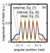
Fig. 3. (Color online) (a) Near-field imaging transformation of the lens. Thick red line: magnitude of H-field illuminating the internal boundary,  $\rho=0.6\,\mu\text{m}$ , in front of the sources. Thin yellow line: the field at the external boundary,  $\rho=3\,\mu\text{m}$ . (b) Thick blue line: impedance matched at the internal boundary. Thin red line: impedance matched at the external boundary. Dashed yellow line: same as the thin yellow line in panel (a).
