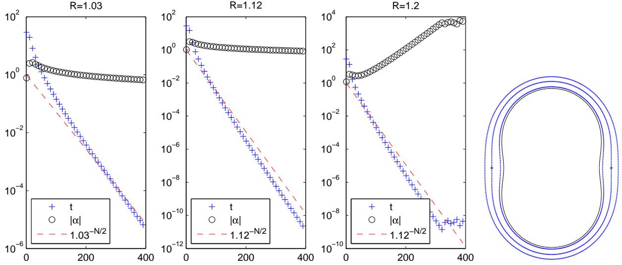
Fig. 9. Left three plots: Estimated (dashed lines) and observed ('+') rates of convergence of the MFS on the inverted ellipse for charge points with conformal radii  $R = 1.03$ ,  $R = 1.12$  and  $R = 1.2$ . The corresponding coefficient norms  $|\alpha|$  are denoted by 'o'. Right plot: Domain and positions of the charge points (shown as dots) for the above three conformal radii, with branch-type singularity locations ('+' signs).
