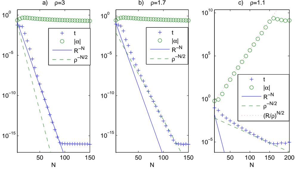
Fig. 3. Convergence and coefficient sizes as a function of  $N$ , for the MFS approximation to the interior Helmholtz BVP in the unit disc given boundary data corresponding to a single source (39) at radius  $\rho$ . The wavenumber is low ( $k = 8$ ). The MFS sources are at  $R = 1.5$ . For visual comparison the relevant power laws from Theorems 3 and 7 are shown (sometimes the constants have been chosen to match the data). There were  $M = 240$  boundary points.
