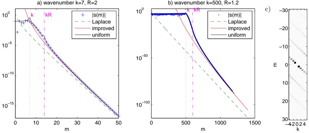
Fig. 2. Comparison for the unit disc of layer-potential eigenvalue magnitudes  $|\hat{s}(m)|$  given in (12) against various asymptotic expressions: ‘Laplace’ (14), ‘improved’ (44), and ‘uniform’ (45). a) low wavenumber, b) high wavenumber. Panel c) shows density plot of matrix elements (20) of  $Q$  for  $N = 10$ , in the domain  $|m| \leq 30$ . In c) we chose unrealistically small values of  $R$  and  $k$  in order to make the super- and sub-diagonals more visible.
