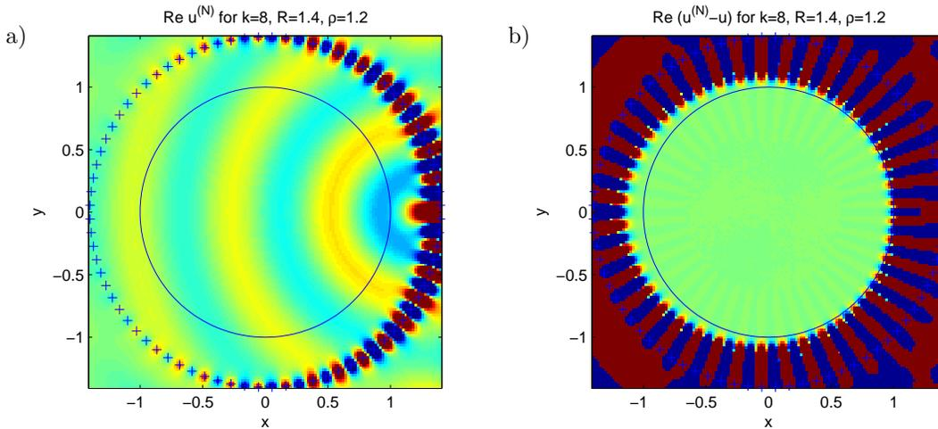
Fig. 4. MFS approximation to the interior Helmholtz BVP in the disc with given boundary data corresponding to a single source (39) outside the domain at  $\rho = 1.2$ , with  $N = 80$  and  $R = 1.4$ . a)  $\text{Re } u^{(N)}$ , b) residual  $\text{Re } (u^{(N)} - u)$  on a color scale  $3 \times 10^4$  times more sensitive than a).
