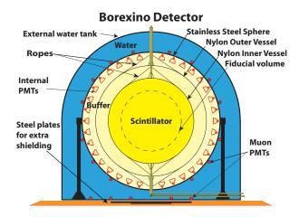
Fig. 2. Schematic drawing of the Borexino detector.
