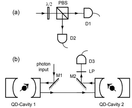
FIG. 3: (a) A proposed setup to measure the giant Faraday rotation and the electron spin polarization.  $\lambda/2$  - wave plate, PBS - polarized beam splitter, D1, D2 - detectors. (b) A proposed scheme to create entanglement between two remote spins via a single photon. Both QD-cavity systems work in the strong-coupling regime. M1, M2 - reflection mirrors, LP - linear polarizer, D3 - detector.
