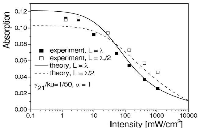
FIG. 8: Intensity dependence of the absorption - at line-center- for a closed transition. The theoretical dependence for  $L = \lambda/2$  is in dashed line, the solid line is for  $L = \lambda$ . The experimental data ( $L = \lambda/2$  : open squares,  $L = \lambda$  : full squares) are for the closed  $F_g = 4 \rightarrow F_e = 5$  transition. For the scale applied to the theoretical curves, see text.
