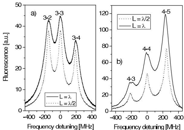
FIG. 5: Illustration of the ETC fluorescence spectra for lower (a,  $7mW/cm^2$ ) and higher (b,  $130mW/cm^2$ ) light intensities at the two studied cell thicknesses.  $Cs$  source temperature:  $127^\circ C$  (a) and  $105^\circ C$  (b).
