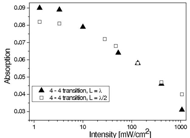
FIG. 4: Experimental absorption at the line center of the  $F_g = 4 \rightarrow F_e = 4$  h.f.s. component, as a function of the irradiating intensity for  $L = \lambda/2$  and  $L = \lambda$ .
