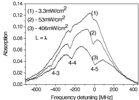
FIG. 3: Absorption spectra across the  $F_g = 4 \rightarrow F_e = \{3, 4, 5\}$  transitions for various intensities (as indicated) at  $L = \lambda$ .
