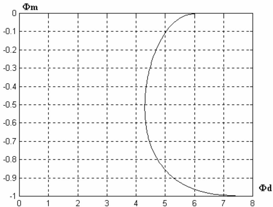
**Fig. 2** The dependence between  $\Phi_d$  and  $\Phi_m$  when  $J_0 = 16$  and the mode is that of unlimited beam.
