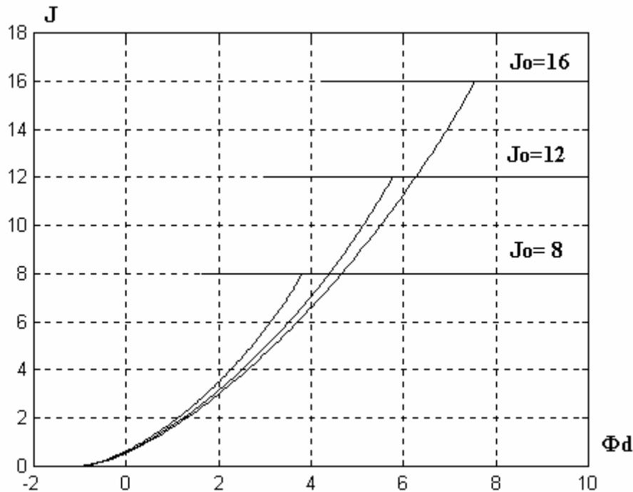
**Fig. 4** Volt-ampere characteristics of a planar vacuum diode for different values of the saturation current.
