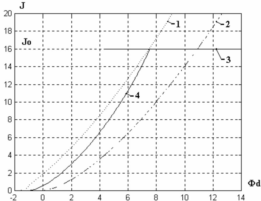
**Fig. 3** Volt-ampere characteristics of the diode when  $J_0 = 16$ : curve 1 - according to (16); curve 2 - according to (17); curve 3 - according to (10); curve 4 - according to (14).
