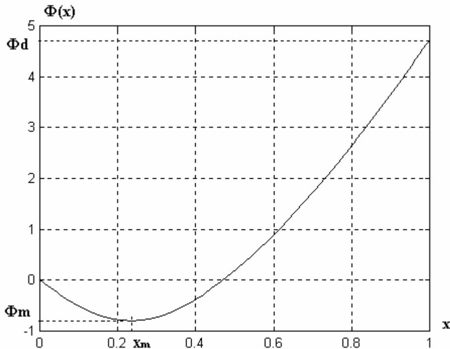
Fig. 1 Dependence of the electrical field potential on the x coordinate when  $J_0=16$  and  $\Phi_m=-0.8$ .
