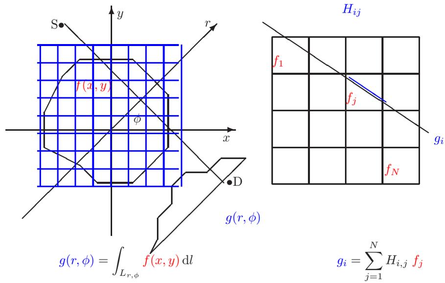
Figure 4: Discretized 2D X ray computed tomography
