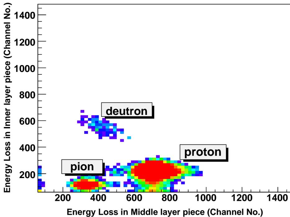
Fig. 10. A two dimensional spectrum of the energy losses in inner and middle layer pieces of ENSTAR mounted at the focal plane exit of Big Karl magnetic spectrograph in  $\Delta E1 - \Delta E2$  configuration. The spectrum shows the pions, protons and deuterons of energies  $\sim 430$  MeV,  $\sim 150$  MeV and  $\sim 80$  MeV respectively, which are selected by a BigKarl momentum setting of 550 MeV/c.
