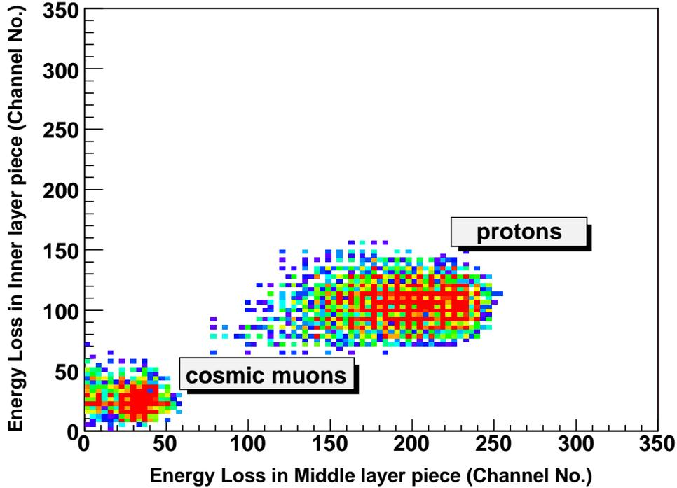
Fig. 11. A two dimensional spectrum of one of the inner layer piece vs the corresponding middle layer piece of ENSTAR for protons in the energy range of 225-330 MeV obtained from pp elastic scattering data. Cosmic ray data from a different run are also shown in the same figure.
