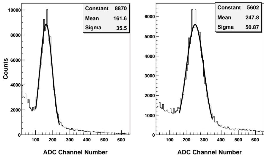
Fig. 12. ADC spectra of two adjacent middle layer scintillators uniformly illuminated in  $\phi$ - direction by scattered particles from beam impinging on a thick target kept in front of detector. Peak positions are used to get the relative gains of various pieces in  $\phi$ -direction.
