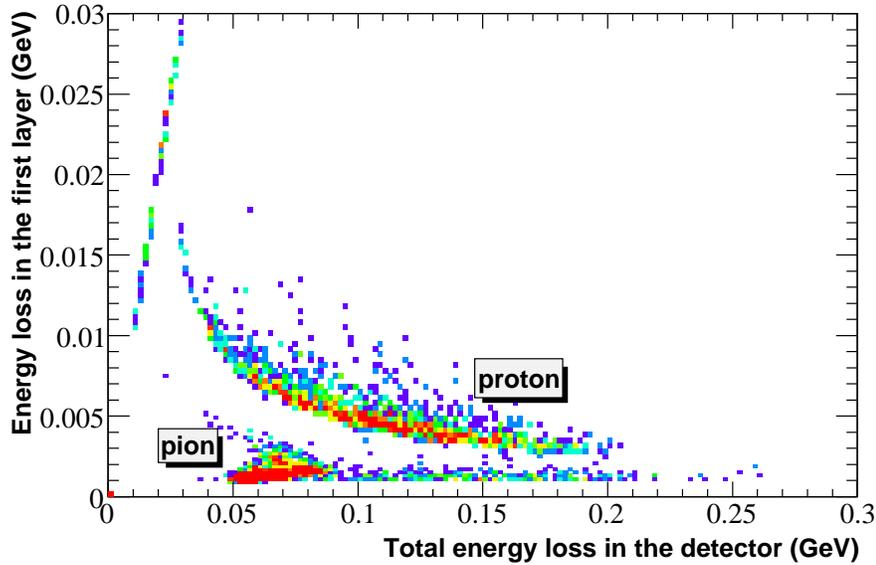
Fig. 6. A two dimensional plot of  $\Delta E$  (energy loss in the inner layer) vs  $E + \Delta E$  (energy loss in all the layers) showing the particle separation in ENSTAR. The results are obtained from GEANT simulations for the events from the  $\eta$ -mesic nucleus decay.
