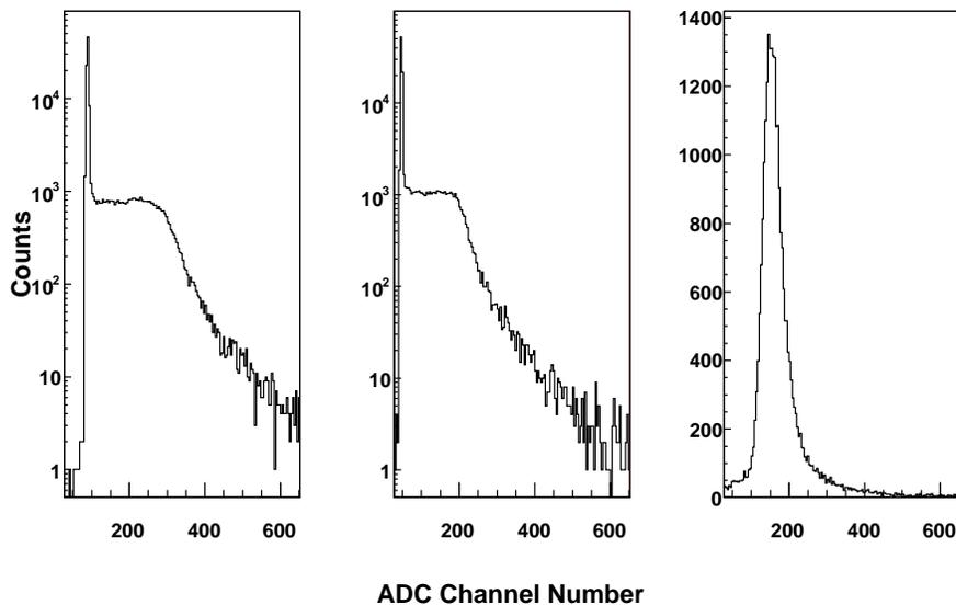
Fig. 13. ADC spectra from two adjacent middle layer scintillators for cosmic ray
