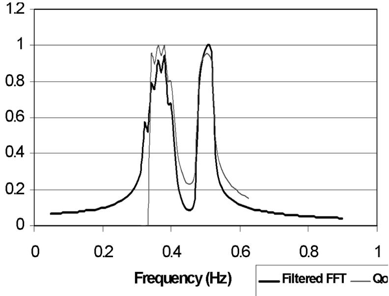
Fig. 13. Filtered FFT of the forcing wave signal of figure 11 with a running mean of 0.04 Hz and the corresponding  $Q_0(T)$  curve; each curve is normalized with respect to its maximum.
