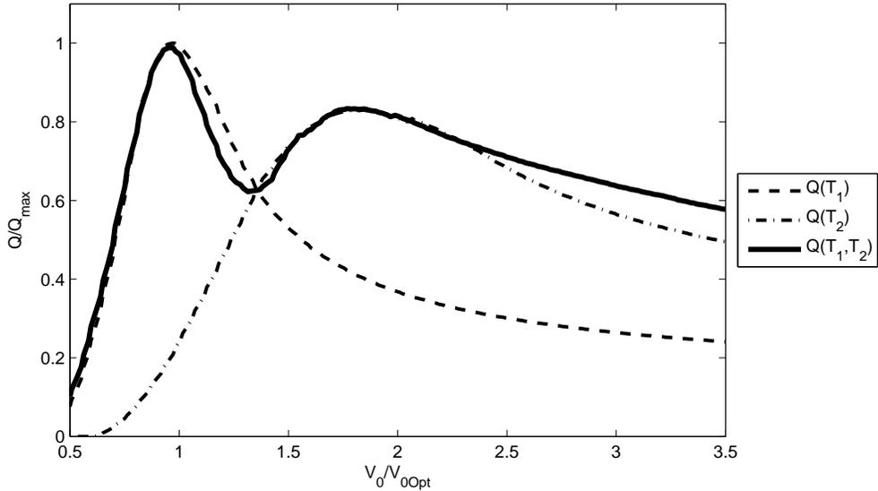
Fig. 10. Flow vs. volume of air in the compression chamber obtained with the numerical model forced by: a signal with components of 2 and 2.6 s ( $Q(T_1, T_2)$ ); only the 2s component ( $Q(T_1)$ ); only the 2.6s component ( $Q(T_2)$ ).
