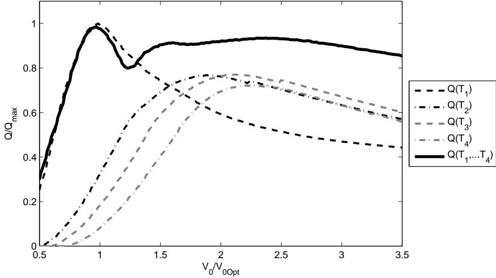
Fig. 12. Flow vs. volume of air in the compression chamber obtained with the numerical model forced by: a signal with components of  $T_i = 2, 2.6, 2.75$  and  $2.9$  seconds (solid line,  $Q(T_1, \dots T_4)$ ) and four series obtained with monochromatic forcings for each component ( $Q(T_i)$ ).
