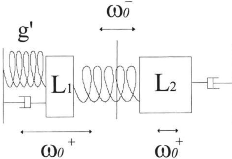
Fig. 2. Representation of the pump as a damped two-mass two-spring oscillator (from Czitrom et al., 2000b)
