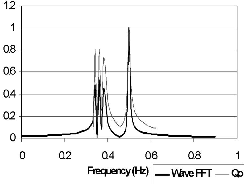
Fig. 11. Fast Fourier Transform of the forcing wave signal and the corresponding graphic for  $Q_0(T)$  for a four-component wave (of 2.9, 2.75 and 2.6 and 2 seconds). Each curve is normalized with respect to its maximum.
