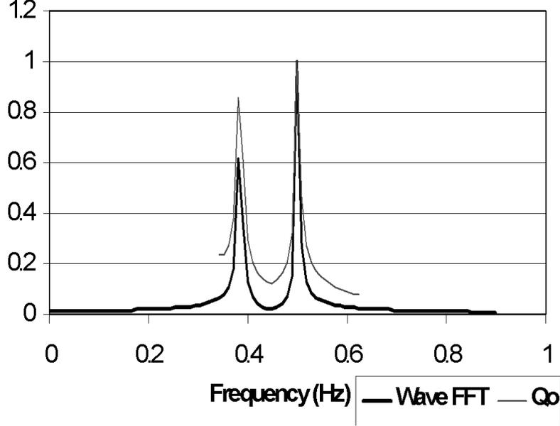
Fig. 9. Fast Fourier Transform of the forcing wave signal and the corresponding graphic for  $Q_0(T)$  for a two-component forcing wave (of 2 and 2.6 seconds periods). Each curve is normalized with respect to its maximum.
