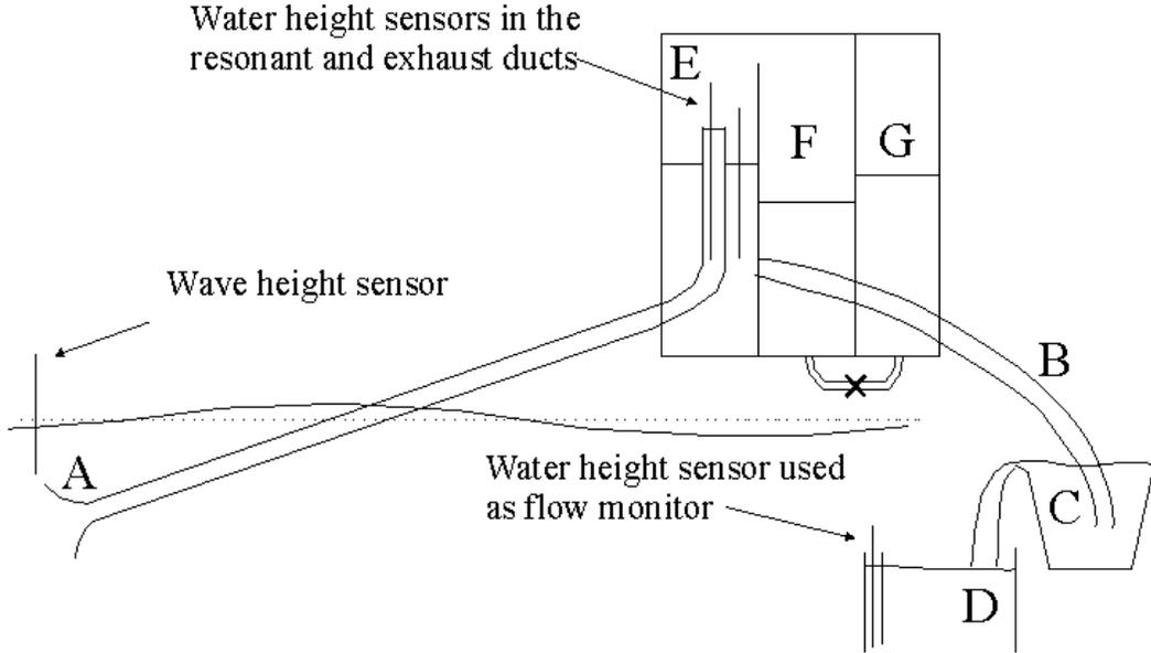
Fig. 4. Schematic diagram of the scale model tested in the wave tank (see text).
