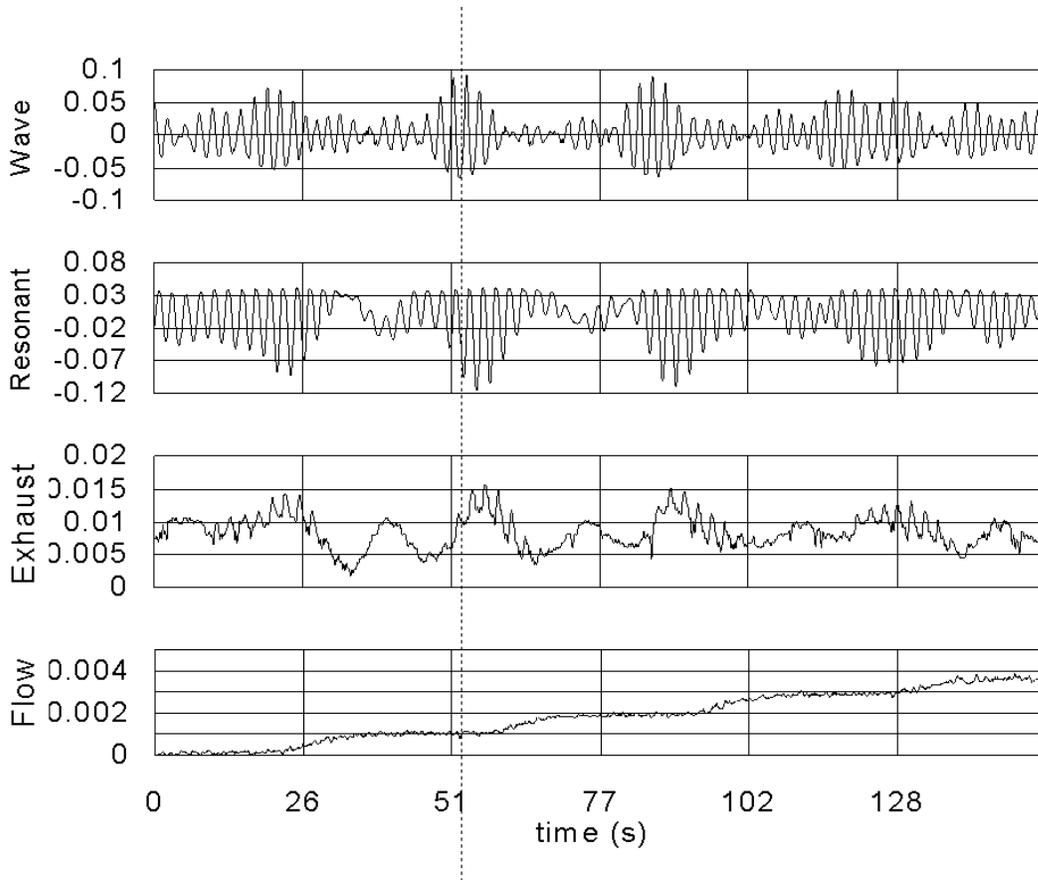
Fig. 5. Time series of the water height measurements in the wave tank, the resonant and exhaust ducts (in metres) and the flow recipient (in cubic metres).
