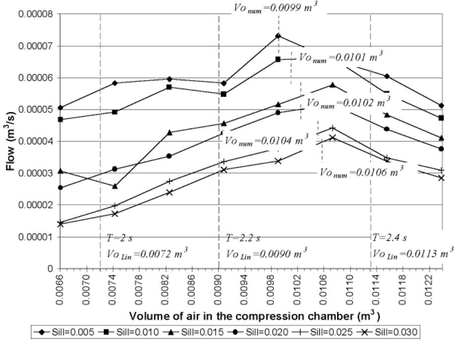
Fig. 8. Average flow rate obtained in the experiments vs. volume of air in the compression chamber for the same forcing wave of figure 7. The long vertical lines show the linearized model prediction  $V_{O_{Lin}}$  for each component. The short vertical lines show the numerical model prediction  $V_0$  for the greater period and each sill height (given in meters).
