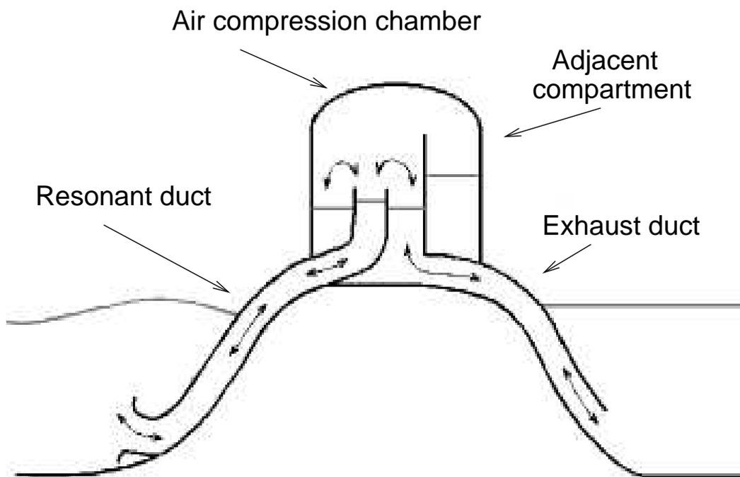
Fig. 1. Schematic diagram of the seawater pump (from Czitrom et al., 2000b)
