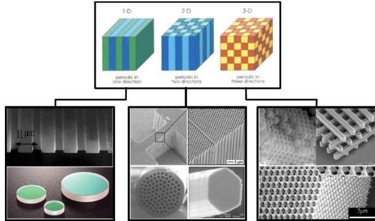
Fig. 1. Examples of one-, two-, and three-dimensional photonic crystals<sup>1-4</sup>.
