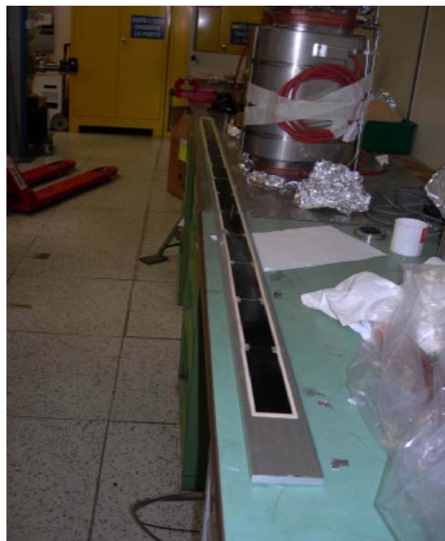
Fig. 14 The ion clearing electrode removed from the wiggler vacuum chamber.
