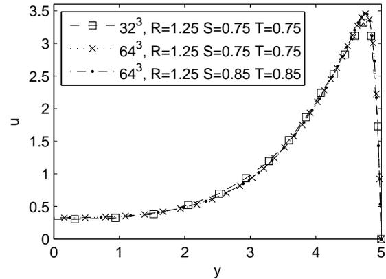
Figure 3: span-wise profile of the stream-wise velocity computed at different grid parameters:  $N_x \times N_y \times N_z = 32 \times 32 \times 32$  (squares) and  $64 \times 64 \times 64$  (crosses and dots),  $(R, S, T) = (1.25, 0.75, 0.75)$  (squares and crosses) and  $(1.25, 0.85, 0.85)$  (dots). Other parameters are common:  $Re = 100$ ,  $N = 16$ ,  $x = 0$ ,  $z = 0$ .
