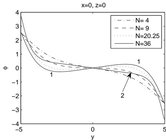
Figure 11: Simulated span-wise electric potential profiles in the center of the magnetic gap ( $x = 0$  and  $z = 0$ ),  $Re = 400$  and  $N = 4$  (dot-dashed),  $N = 9$  (dashed),  $N = 20.25$  (dotted),  $N = 36$ , experimental magnetic field (solid line 1) and  $N = 36$ , simplified field (solid line 2).
