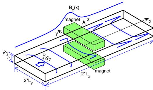
Figure 1: Coordinate system and sketch of the problem: rectangular channel  $2L_x \times 2L_y \times 2L_z$  and two magnets on the bottom and top walls. Qualitatively, there are shown transverse magnetic field  $B_z(x)$  varying along stream-wise direction, and span-wise profile of stream-wise velocity  $u_x(y)$ . The center of the coordinate system is in the center of the magnetic gap.
