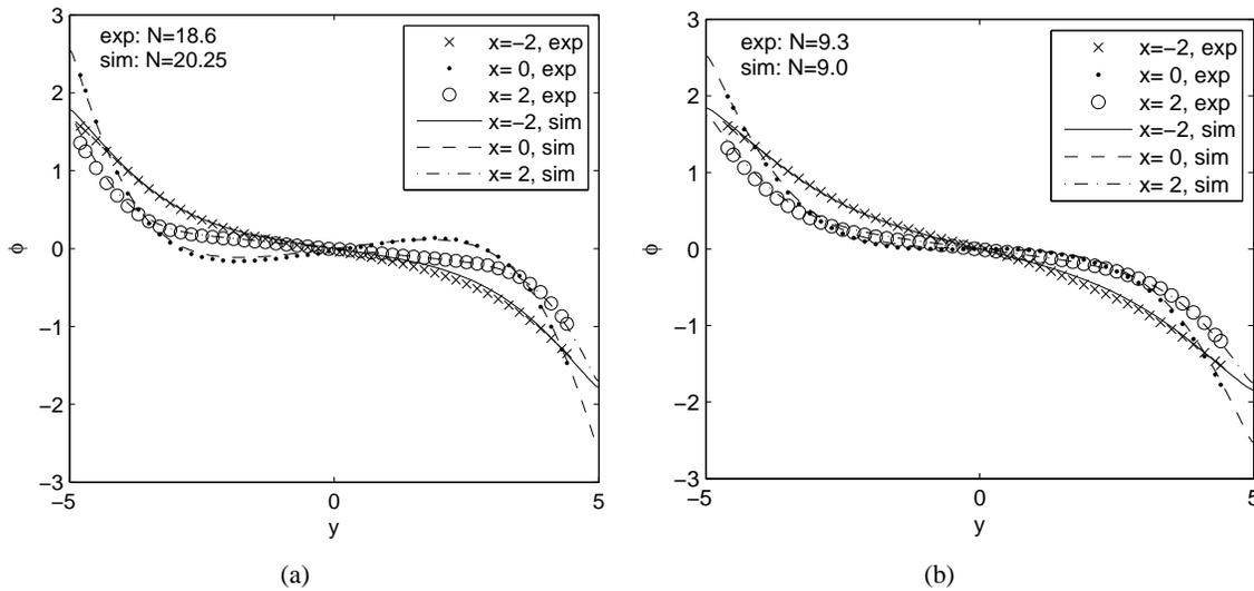
Figure 12: Experimental (symbols) and simulated (lines) span-wise electric potential profiles at  $z = 0$  and  $x = -2$  (crosses and solid lines), 0 (dots and dashed lines), 2 (circles and dot-dashed lines). Plot *a* is for  $N \approx 20$ :  $(Re, N) = (2000, 18.6)$  (experiment) and  $(Re, N) = (400, 20.25)$  (simulation). Plot *b* is for  $N \approx 9$ :  $(Re, N) = (4000, 9.3)$  (experiment) and  $(Re, N) = (400, 9)$  (simulation).
