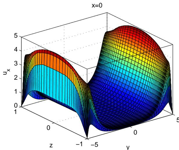
Figure 5: 3D M-shaped velocity profile,  $x = 0$ ,  $Re = 400$ ,  $N = 36$
