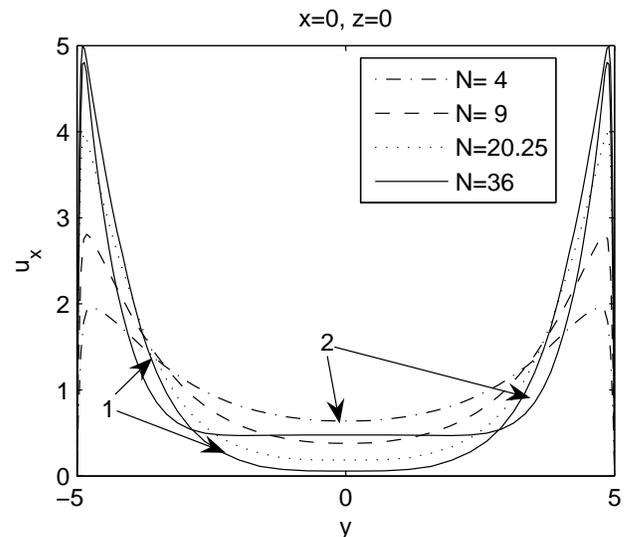
Figure 6: Stream-wise velocity profiles in span-wise direction in the center of the magnetic gap ( $x = 0$  and  $z = 0$ ),  $Re = 400$  and  $N = 4$  (dot-dashed),  $N = 9$  (dashed),  $N = 20.25$  (dotted),  $N = 36$ , experimental field (solid line 1) and  $N = 36$ , simplified field (solid line 2).
