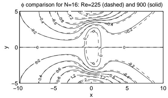
Figure 10: Electric potential distribution,  $\phi(x,y)$  in central horizontal plane ( $z = 0$ ) for  $N = 16$ , simulation:  $Re = 900$  (solid) and  $Re = 225$  (dashed).
