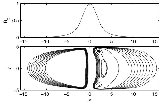
Figure 16: Electric current paths in the central horizontal plane ( $z = 0$ ) under the experimental magnetic field,  $Re = 400$ ,  $N = 36$ . The lines are not equidistant since they were obtained by integration from a few starting points at  $(x, y) = (-0.5, 0), (0.5, 0), (2.1, 4.1), (2.1, -4.1)$ .
