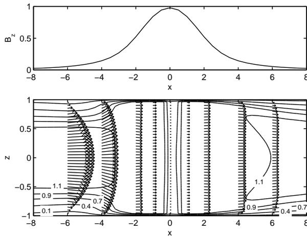
Figure 9: Vector plot of the velocity components  $u_x$  and  $u_z$  in the central vertical plane at  $y = 0$ ,  $Re = 400$ ,  $N = 36$ . The isolines are plotted at constant level of the normalized vertical profile  $p(z;x)$  and give additional information about the flatness of the velocity profile.
