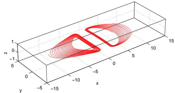
Figure 18: 3D electric current path for the simplified magnetic field without span-wise dependence.
