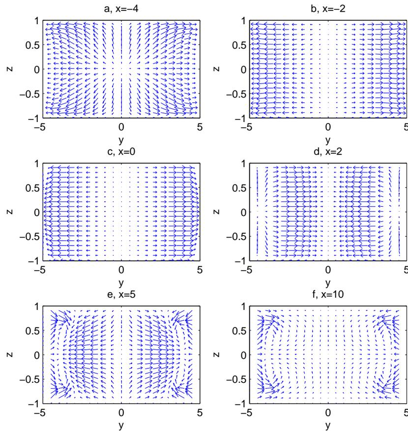
Figure 8: Vector plots of the vertical and span-wise velocity components at the following vertical sections of the channel: (a)  $x = -4$ , (b)  $x = -2$ , (c)  $x = 0$ , (d)  $x = 2$ , (e)  $x = 6$ , (f)  $x = 11$  at  $Re = 400$ ,  $N = 36$ . An interesting feature is the swirling flow that arises in the corners behind the magnet (plot  $e, f$ ).
