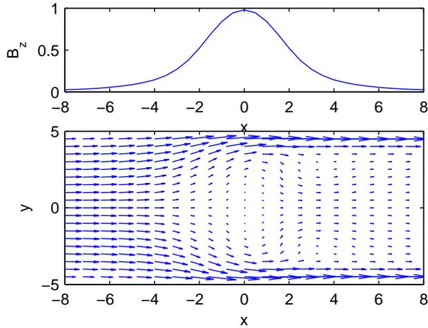
Figure 7: Vector plot of the velocity field in the central horizontal plane,  $z = 0$ . The upper part shows the intensity of the magnetic field on the straight line  $z = 0$ ,  $y = 0$ ,  $Re = 400$ ,  $N = 36$ .
