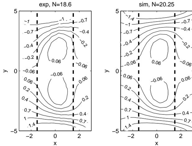
Figure 13: Electric potential distribution,  $\phi(x,y)$ , in the central horizontal plane ( $z = 0$ ) for  $N \approx 20$ : experiment,  $Re = 2000, N = 18.6$  (left) and simulation  $Re = 400, N = 20.25$  (right). Bold dashed lines are physical borders of the magnetic gap.
