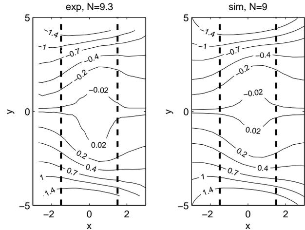
Figure 14: Electric potential distribution,  $\phi(x,y)$  in central horizontal plane ( $z = 0$ ) for  $N \approx 9$ : experiment,  $Re = 4000, N = 9.3$  (left) and simulation  $Re = 400, N = 9$  (right). Bold dashed lines are physical borders of the magnetic gap.
