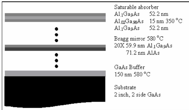
**Fig. 1** MQW structure, mirror design to work around 850 nm and absorber at 850 nm, labelled IV in figure 3.
