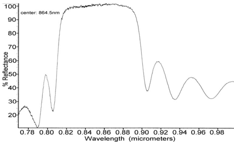
**Fig. 2** Reflectance at low intensity for the MQW of figure 1.
