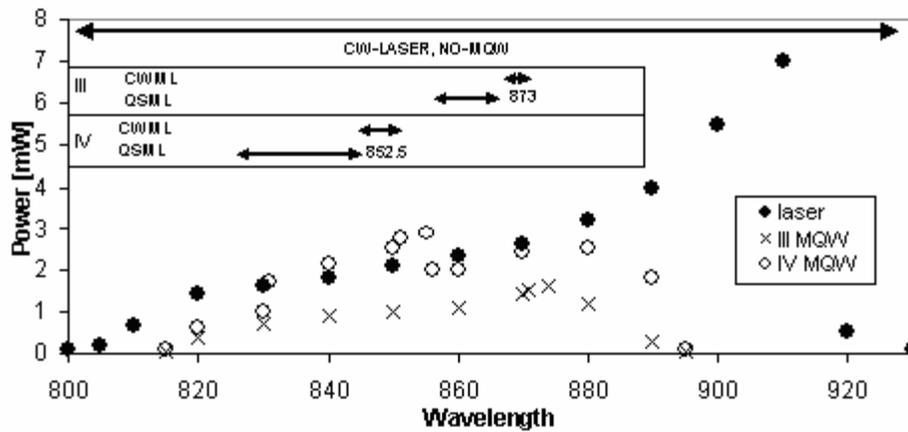
**Fig. 3** Behaviour of a LiSAF laser without MQW, and with two designs of MQW.
