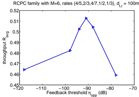
Fig. 4. Throughput as a function of feedback threshold.
