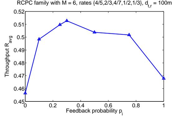
Fig. 3. Throughput as a function of feedback probability.
