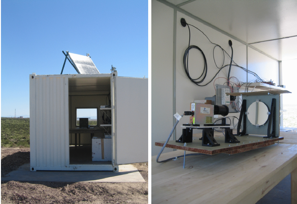
Fig. 2. Photos of the enclosure (left) and the light source (right) at the Los Morados APF facility. In the photograph on the left, the Los Morados FD can be seen on the horizon (to the left of the container).
