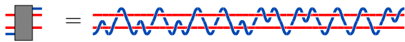
FIG. 4: An example of an injection weave for the Fibonacci anyon model ( SO(3)_3 or SU(2)_3 ). This injection was first discussed in Ref. 7 and approximates the identity operation on the Hilbert space to better than one part in 10^2 , while transferring the warp quasiparticle from the bottom to the top. Longer weaves will approximate the identity exponentially more closely with the weave becoming longer only linearly [7, 16]. The box on the left establishes the notation used in Fig. 5 below.
