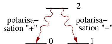
**Figure 7.1:**  $\Lambda$ -level configuration of the dipole source with the two degenerate ground states  $|0\rangle$  and  $|1\rangle$ , the excited state  $|2\rangle$  and optical transitions corresponding to the two orthogonal polarisations “+” and “-”
