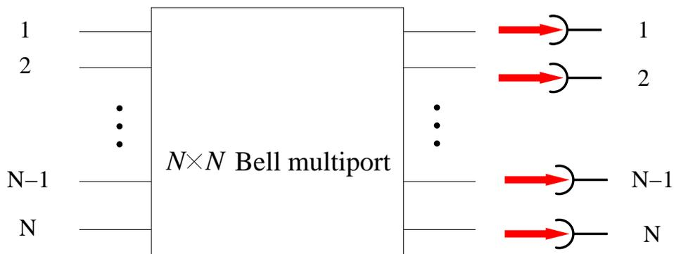
**Figure 2.1:** Experimental setup for the generation of multiphoton entanglement by passing  $N$  single photons through an  $N \times N$  Bell multiport beam splitter. The state preparation is considered successful under the condition of the collection of one photon per output.
