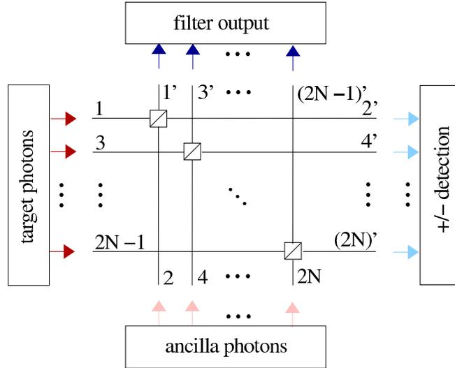
**Figure 4.2:** Experimental setup for the realisation of the  $N$ -photon quantum filter (4.2). The  $N$  polarising beam splitters each compare the state of one of the target photons with the state of one of the ancilla photons, which are initially prepared in the GHZ state  $|A^{(N)}\rangle$ . Besides,  $N$  detectors perform photon measurements in the polarisation basis (4.8). The output photons leave the system via the odd numbered output ports.
