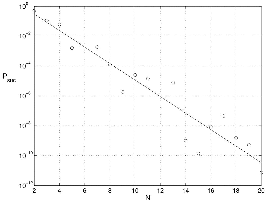
**Figure 2.3:** The success rate for the generation of  $N$ -photon  $W$ -states  $P_{\text{suc}}$  as a function of  $N$ . The solid line approximates the exact results via the equation  $P_{\text{suc}} = e^{a-bN}$  with  $a = 1.35 \pm 1.32$  and  $b = 1.27 \pm 0.10$
