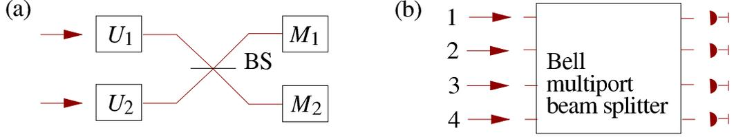
**Figure 5.3:** Linear optics networks for the realisation of a measurement of the basis states  $|\Phi_i\rangle$  defined in Sections (5.2.4,5.2.5) after encoding the photonic qubits in the polarisation degrees of two photons (a) or into four different spatial photon modes (b) involving either a beam splitter (BS) or a  $4 \times 4$  Bell multiport beam splitter.
