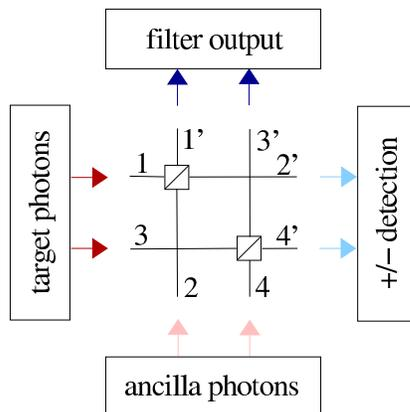
**Figure 4.1:** Experimental setup for the realisation of a 2-photon parity filter. The target photons enter the setup via the input modes 1 and 3, while the ancilla photons enter the setup via inputs 2 and 4. Within the setup, each photon has to pass one polarising beam splitter. Under the condition of the detection of one photon in each of the outputs 2' and 4', the filter succeeded and the projected output state leaves the system via the modes 1' and 3'.
