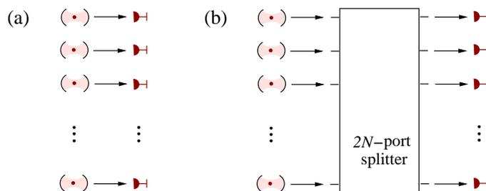
**Figure 6.1:** Experimental setup. (a) During the final “*push button*” step, the entanglement of  $N$  atom-cavity systems is mapped onto the state of  $N$  newly generated photons. (b) The initialisation of the system requires postselective measurements on the photon emission from the  $N$  cavities through a multiport beamsplitter.
