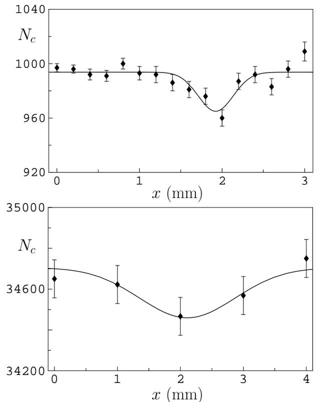
FIG. 2: Number of coincidences  $N_c$  as a function of the path difference  $x = S_{D1} - S_{D2}$  of the detectors from the splitter. Above: scintillator detectors, translation step  $0.2 \text{ mm}$ ; below: gas detector, translation step  $1 \text{ mm}$ . The dip appears at  $x_0 \simeq 2 \text{ mm}$  due to calibration. The parameters  $\tau_D, \tau_c, N_c^{(\infty)}$  and  $x_0$ , by substituting  $t = (x - x_0)/v$  in Eq. (9), are determined by a best fit (see text).
