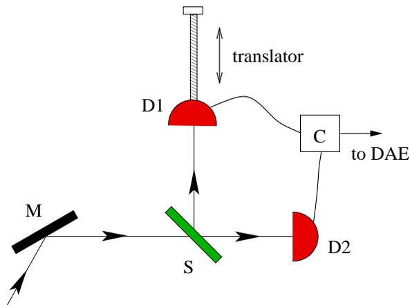
FIG. 1: Schematic drawing of the experimental setup: M=monochromator, S=beam splitter,  $D_{1,2}$ =detectors, C=coincidence counter, DAE=Data Acquisition Electronics. The two detectors can be positioned at the same distance from S, and one of them can be moved across this distance. The collimators are not shown.
