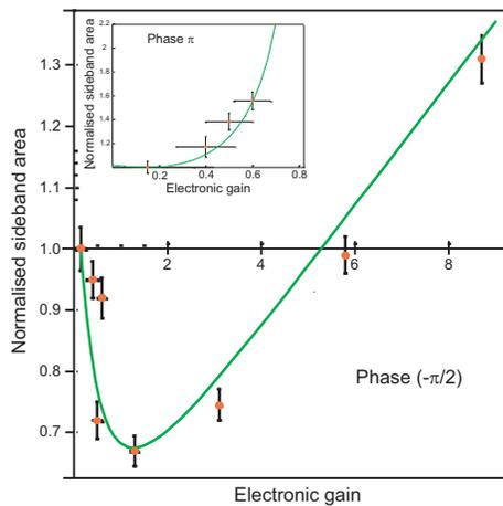
FIG. 3: Steady-state energy of the cooled oscillator: measured sideband area, normalized to the value without feedback, versus gain of the feedback loop, for  $(-\pi/2)$  (a) and  $\pi$  (b) feedback phase. The curves are the model calculations. The gain axis is scaled to the experimental values of the electronic gain.
