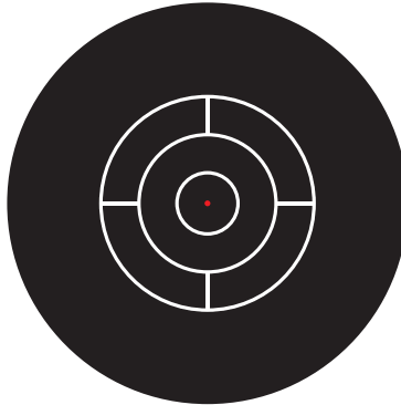
FIG. 4: Test trap with total diameter of 35 mm. Black regions denote electrodes and white regions denote isolating surface. As said before the isolating surface has been mostly covered by electrodes to avoid charging up. This configuration has three active electrodes plus an external grounded one. The red circle in the center is a hole through which electrons are loaded from the rear side.
