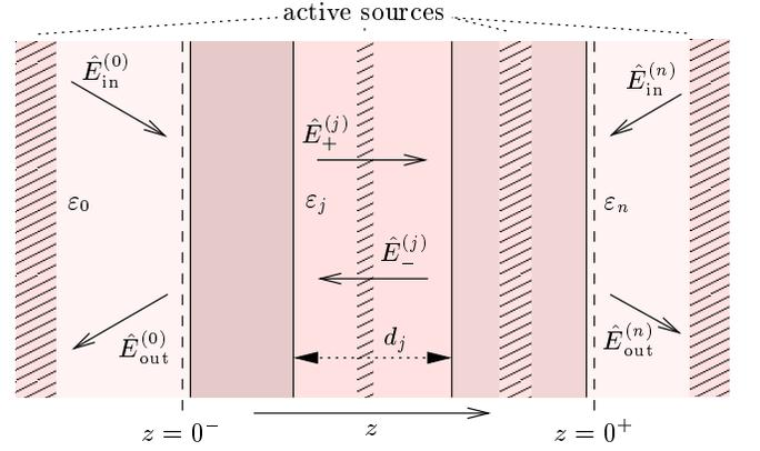
FIG. 1: Scheme of the multilayer dielectric plate. The hatched regions indicate the presence of active light sources.
