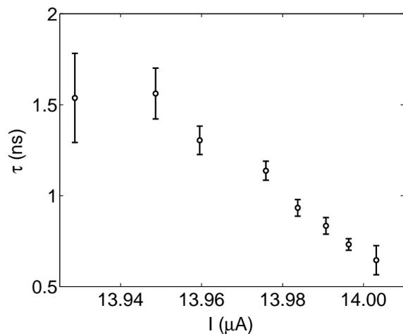
FIG. 5: Coherence time  $\tau$  vs. bias current,  $I$ . Note that the escape rate from the ground state at  $13.93 \mu\text{A}$  is around  $10^3/\text{s}$  while at  $14.01\mu\text{A}$ , it is around  $3 \times 10^6/\text{s}$ .
