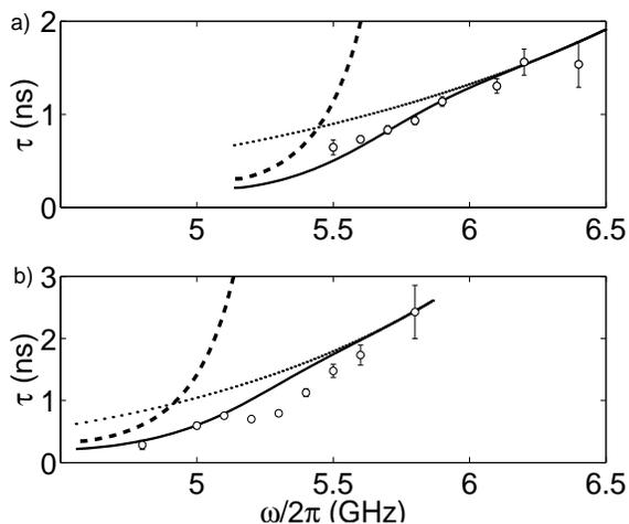
FIG. 6: Coherence time,  $\tau$ , vs. bias current  $I$ . Solid lines are the theoretical fit for each data set. Lower frequency corresponds to larger current. The parameters for the fit in (a) are  $I_0 = 14.12 \mu A$  and  $C = 3.7 pF$ . For the fit in (b)  $I_0 = 10.645 \mu A$  and  $C = 3.7 pF$ . The dashed lines represent the contribution from the escape rate, and the dotted lines the contribution from current noise.
