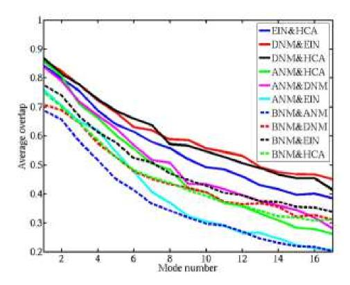
Figure 3: Overlap scores for normal modes from different potentials averaged over all 83 structures. Each curve is a comparison between a pair of potentials over the 17 lowest frequency modes. The solid curves compare different ENM-like potentials, while the dotted curves compare CHARMM-based BNM results with those from ENM potentials.
