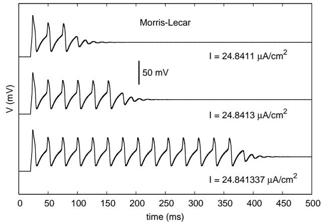
FIG. 2: Examples of transient behavior near  $I_c$  for the ML system. The constant step current is applied at  $t = 10$  ms. The estimated critical current is  $I_c = 24.84134676279 \mu\text{A}/\text{cm}^2$  for an integration time step  $dt = 0.01$  ms.
