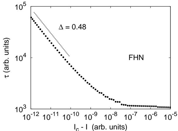
FIG. 6: Relaxation times for the FitzHugh-Nagumo model as a function of the distance to critical current. Note that the power law becomes visible only *very* close to the fold bifurcation ( $I_c - I \sim 10^{-9}$ ).
