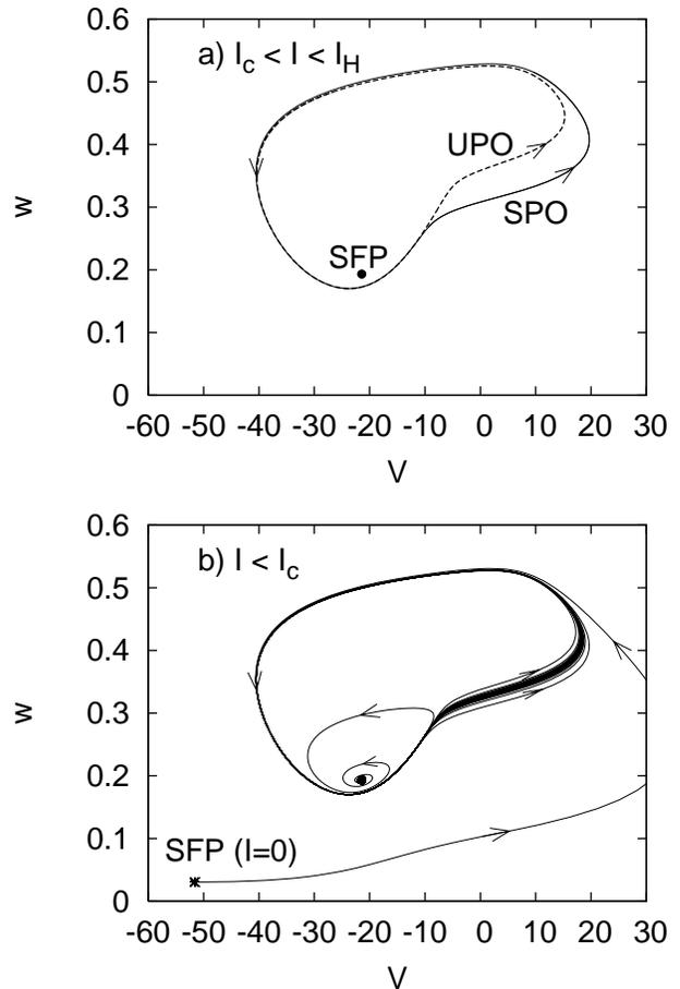
FIG. 7: Phase portraits of the ML model for  $I$  slightly above (a) and below (b)  $I_c$ . The long transient is dominated by the time it takes to pass through the region where the limit cycles are about to emerge. SPO (UPO) = Stable (Unstable) Periodic Orbit, SFP = Stable Fixed Point. Horizontal axes ( $V$ ) in mV and vertical axes ( $W$ ) are dimensionless.
