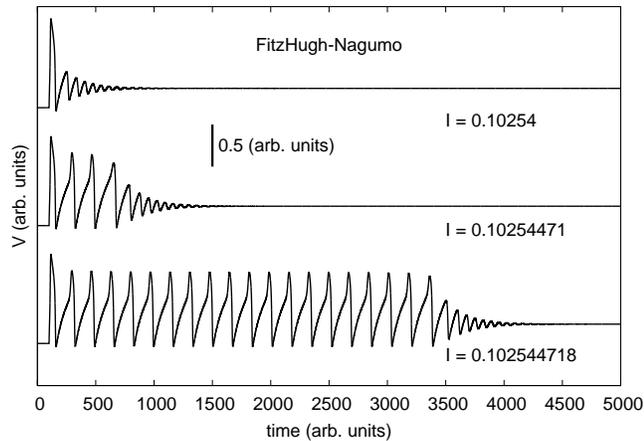
FIG. 3: Examples of transient behavior near  $I_c$  for the FHN system. The constant step current is applied at  $t = 10$ . The estimated critical current is  $I_c = 0.1025447183127$  for an integration time step  $dt = 0.01$  (all quantities in arbitrary units).
