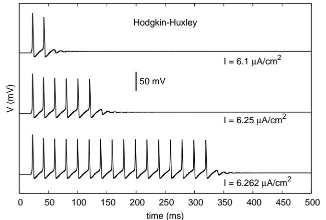
FIG. 1: Examples of transient behavior near  $I_c$  for the HH model. The constant step current is applied at  $t = 10 \text{ ms}$ . The estimated critical current is  $I_c = 6.26422125685 \mu\text{A}/\text{cm}^2$  for an integration time step  $dt = 0.01 \text{ ms}$ .
