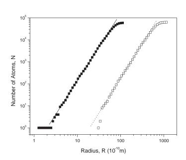
FIG. 2: A typical log-log plot of the number of atoms versus the radius for the 23S rRNA ( $\blacksquare$ ) and the 50S subunit ( $\Box$ ). The least-square fits on the slope of the 23S rRNA (solid line) and the 50S subunit (dotted line) yield 3.01 and 3.06, respectively. The plot for the 50S subunit is shifted to the right by the factor of 10 for the display purpose.
