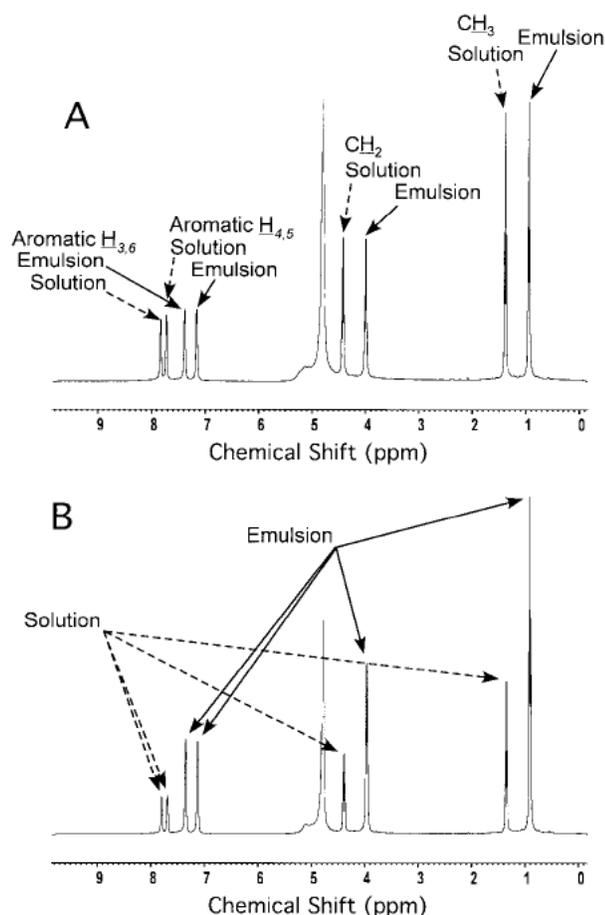
FIG. 8:  $^1\text{H}$  NMR spectrum of an emulsion of DEP in  $^2\text{H}_2\text{O}$ . For resonance assignments, the basis of which is discussed in the text, see Fig. 6(A). The solid arrows indicate resonances from DEP in the emulsion phase. The broken arrows indicate resonances from DEP in aqueous solution. (A) Overall concentration of DEP was  $10\text{ mmol L}^{-1}$ . (B) Overall concentration of DEP was  $15\text{ mmol L}^{-1}$ .
