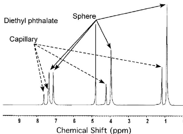
FIG. 7: <sup>1</sup>H NMR spectrum of neat DEP in a glass *cs* assembly (see Fig. 3) with <sup>2</sup>H<sub>2</sub>O in the NMR tube. The resonances from DEP in the glass sphere of the *cs* are indicated by solid arrows, whereas resonances from DEP in the cylindrical capillary are indicated by the broken arrows.
