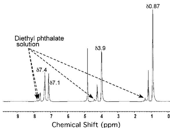
FIG. 9:  $^1\text{H}$  NMR spectrum of  $15 \text{ mmol L}^{-1}$  DEP in  $^2\text{H}_2\text{O}$  in a 10-mm NMR tube with neat DEP in the *cs* assembly. The resonances from the DEP in the aqueous phase, i.e., in solution, are indicated by the broken arrows, while the assignments of the other resonances are described in the text.
