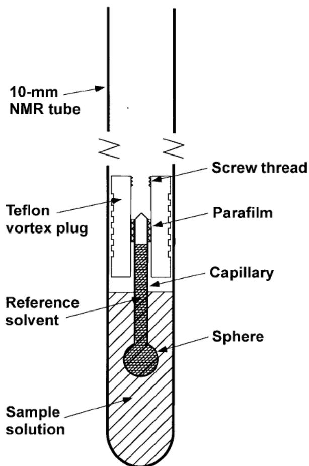
FIG. 3: Capillary-sphere (cs) assembly for the measurement of magnetic susceptibility using NMR spectroscopy. The sample solution whose magnetic susceptibility is to be determined is placed in the 10-mm NMR tube before insertion of the cs and vortex plug. The cs contains a reference liquid, such as benzene. The cs is positioned in the sample tube so that signals of similar intensity are obtained from the contents of both the capillary and the sphere.
