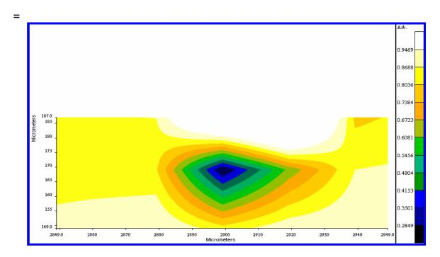
**Fig. 4.1.3**. Spatial Resolution Test: FT-NIR Reflection Mode Image of a 1 cm, Cubic Zirconium Single Crystal at a resolution of  $\sim 1$  micron (Plot of the band ratio: 7253 to 5485 cm<sup>-1</sup>).
