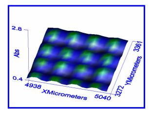
**Fig. 4.1.1.** FT-IR Single Wavenumber (761 cm<sup>-1</sup>) Chemical Images of 6 micron diameter Latex Beads placed on an electron microscope grid. These FT-IR images were obtained with the Spotlight 300 IR-Microspectrometer using a total acquisition time of ~10 minutes, and demonstrate both the high imaging speed and the maximum microscopic resolution of this novel-design instrument.
