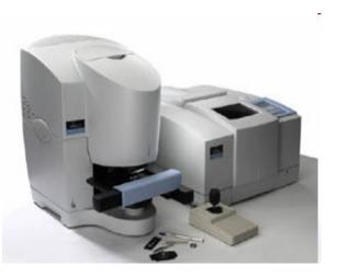
Fig. 3.2.1. FT-IR Microspectrometer (Spotlight 300) introduced by the PerkinElmer Co.
