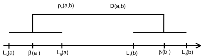
FIG. 5: Eight quantities characterize a loop stitch.
