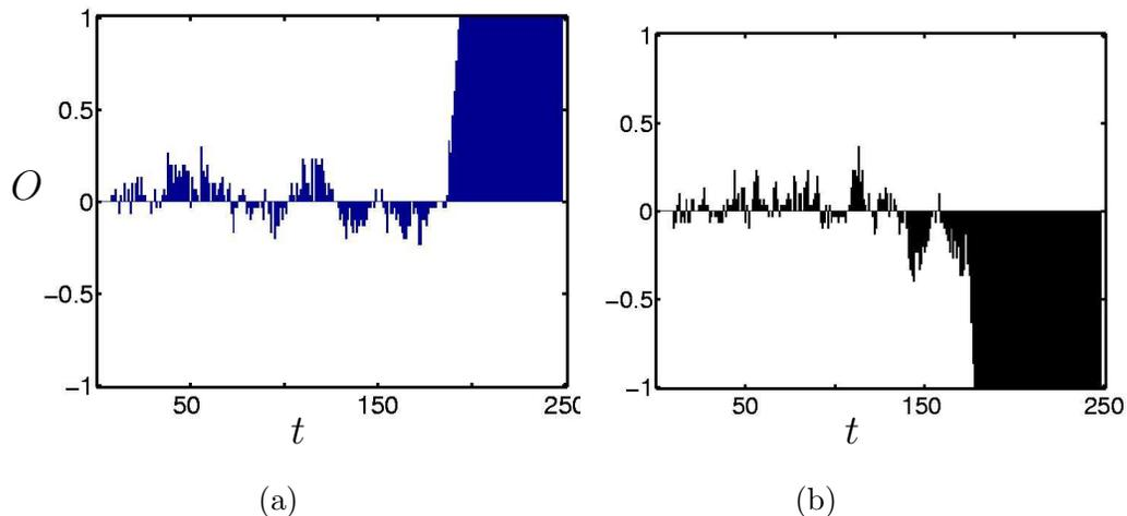
Fig. 21. Evolution of the global order parameter,  $O$ , showing the formation of the vortex (a) in CW direction ( $O \rightarrow +1$ ) at  $t \simeq 190$  time steps for parameters,  $N_{\text{tot}} = 30$ ,  $a = 0.7$ , and  $q = 0.16$ , (b) in CCW direction ( $O \rightarrow -1$ ) at  $t \simeq 180$  time steps for the same parameters.
