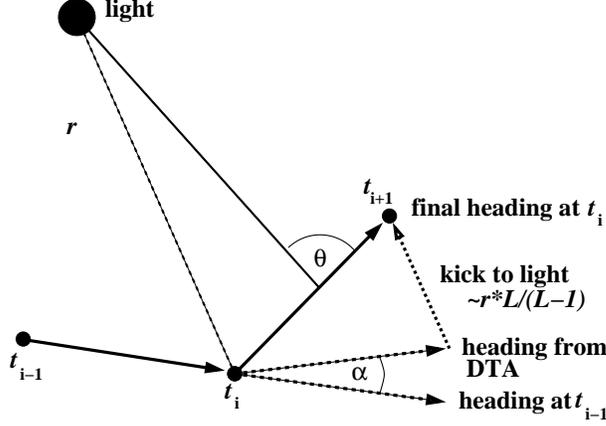
Fig. 17. The geometry of a pair of iterations,  $t_i$  and  $t_{i+1}$ , of the RWT showing distance to the light source  $r$ , heading angle  $\theta$ , and turning angle  $\alpha$ , as taken from the DTA shown in Fig. 16.
